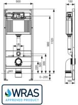
Only for WC pans designed for low volume flushing. Contact Sales Office for latest specifications
