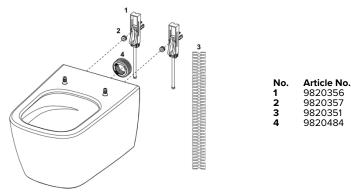
Spare Parts Concealed mounting Knurled nut (2x) for concealed mounting Sound insulation tape Seal for flush pipe connection
