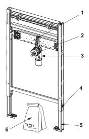
9310004 - TECEprofil washstand module with concealed odour trap, installation height 1120 mm
