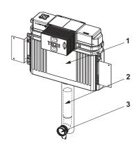
9370500 – TECEbox Octa II cistern, 8 cm, for floor-standing toilet, with reinforcement fabric, installation height 1075 mm
