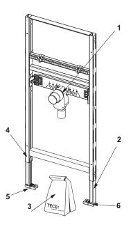
9310019 – TECEprofil washstand module with concealed odour trap, installation height 820-980 mm
