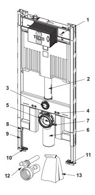
9300501 – TECEprofil toilet module with Octa II cistern, 8 cm, with connection for odour extraction, installation height 1120 mm
