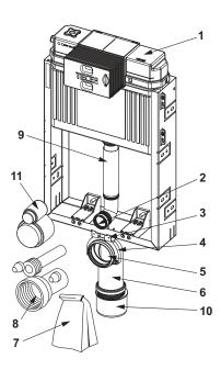
9375300 – TECEbox toilet module with Uni cistern and tile base front, installation height 820 mm
