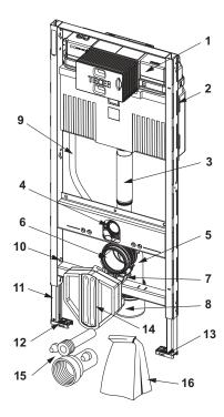
9300302 - TECEprofil toilet module with Uni cistern, installation height 1120 mm
