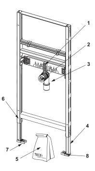
9310018 - TECEprofil washstand module, installation height 820-980 mm
