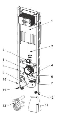
9300102 – TECEprofil toilet module with Uni cistern, with integrated warm and cold water hygiene flushing function, installation height 1120 mm
