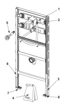
9320010 - TECEprofil urinal module for wall-mounted flush valve, installation height 1120 mm
