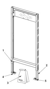
9330000 – TECEprofil bidet module for wall-mounted bidet, installation height 1120 mm 9330005 – TECEprofil bidet module for wall-mounted bidet, installation height 820 mm
