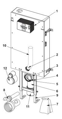
9041308 - TECEbox Uni cistern including mounting plate, installation height 1060 mm
