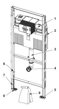
9300600 - TECEprofil toilet module with Compact 320 cistern, installation height 1120 mm
