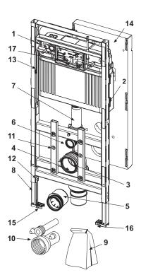
$9600400-{\rm TECE}$  lux toilet module 400, subsequent height adjustment, with odour extraction, installation height 1120 mm
