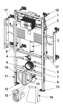
9300303 – TECEprofil toilet module with Uni cistern, with connection for odour extraction, installation height 1120 mm
