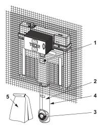
9370501 – TECEbox toilet module with Octa II cistern, 8 cm, for wall toilet, installation height 1075 mm
