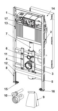
$9600200-\mbox{TECElux}$  toilet module 200, with subsequent height adjustment, installation height 1120 mm
