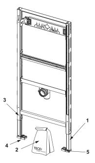
9340000 – TECEprofil bath/shower module for flush-mounted and wall-mounted fittings, installation height 1120 mm
