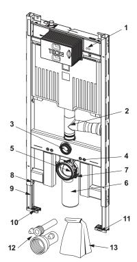
9300502 – TECEprofil toilet module with Octa II cistern, 8 cm, installation height 1120 mm
