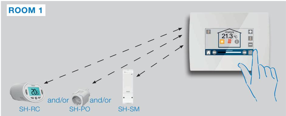
**Warning!** In this installation type, the thermostat (MASTER) must be in regulation Air mode (not floor or Air + Floor)
