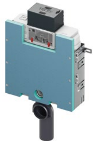
TECEbox toilet module with Uni cistern and tile base front, installation height 820 mm: Toilet module for installation in a bricked-in pre-wall in front of a solid wall, depth-adjustable.
