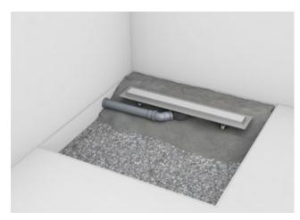
Step 2: The screed is installed with a gradient of 1 to 2% to the channel to ensure optimum drainage.
