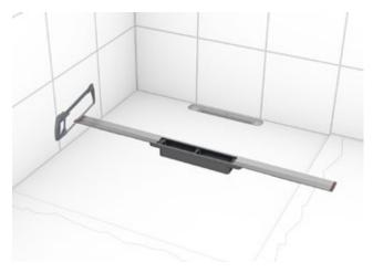
Step 5: The stainless steel is installed recessed and can be shortened on both sides where required. This means it can be precisely tailored to the width of the shower area.
