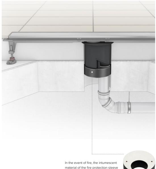
material of the fire protection sleeve expands and closes the drain, safely protecting it from fire and smoke.
