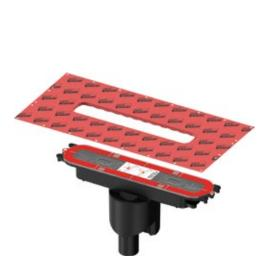
The assortment of drains in the TECEdrainprofile range consists of a flat drain and a "standard" drain. The factory fitted Seal System sealing sleeve is included in the scope of delivery. It seals safe and tight with a simple click. The vertical drain is suitable for all applications when the drain pipe is to be routed vertically through the ceiling. At 47 mm, it is also the flattest in the range.
