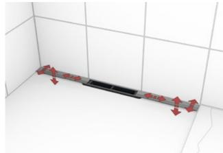
Step 6: The shower profile can still be finely adjusted both horizontally and vertically even after the drain is mounted in the screed and can be adjusted to different thicknesses of wall and floor covers.
