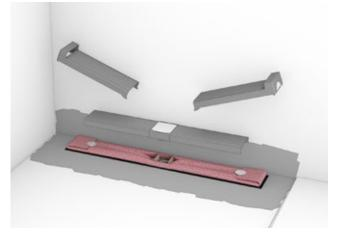
Step 5: After filling with screed, the protective construction cover is removed and the first layer of the composite seal is applied.
