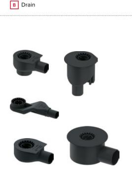
Drains for TECEdrainline shower channels are available in four heights from 53 to 133 mm and as a vertical drain. All drains can be freely combined with all TECEdrainline channels according to the necessary drainage capacity and available installation height.
