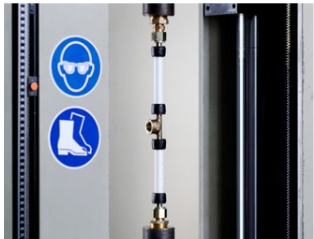
TECElogo-Ax in the pull-out test: tested in the system.
