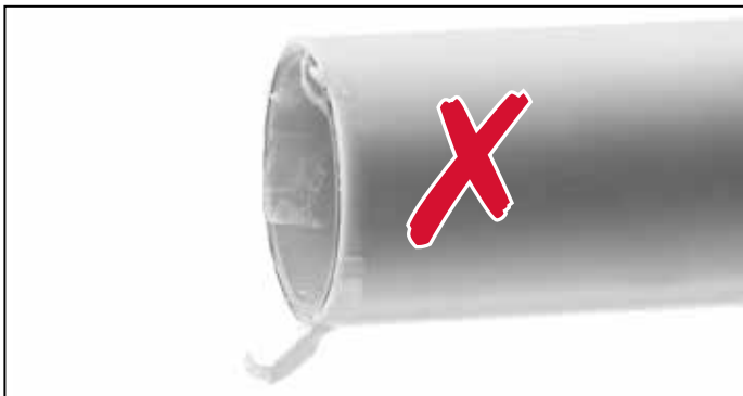
Incorrectly calibrated pipe
