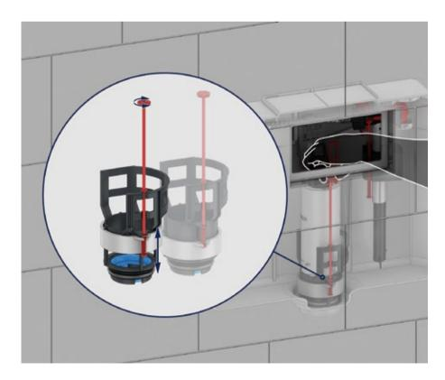
By turning the spindle, the throttle ring moves downwards, thereby reducing the flush flow. In the lowest position, however, a small gap still remains open so that flushing cannot be completely shut off by mistake.
