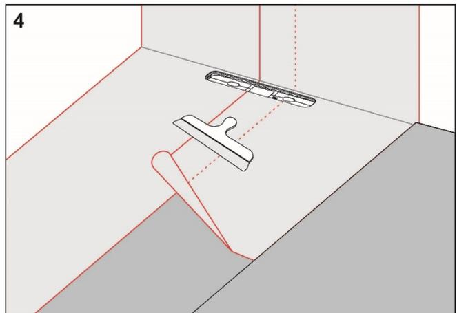
Install Schönox Folie and overlap the drain collar by a minimum of 50 mm. Seal all seams with Schönox iFIX or Schönox HA.
