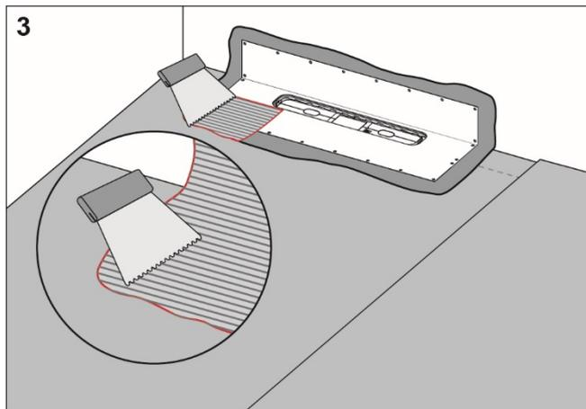
Apply Mapei Mapeguard WP Adhesive on the drain collar and on the rest of the floor and wall area.
