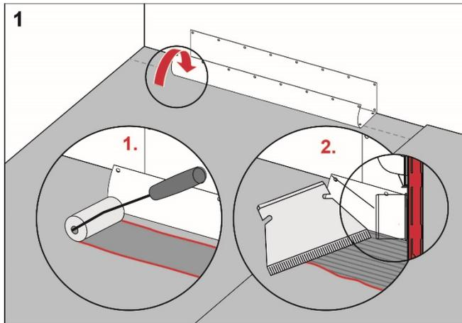
Apply Mapei Mapeguard WP Adhesive on the floor and wall areas which the drain collar will cover. Spread the adhesive with a brush, roller or adhesive spreader.
