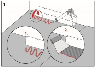
Apply KD+ Skarvlim to the floor and wall areas which the drain collar will cover. Spread the adhesive with a fine-toothed adhesive spreader.
