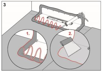
Apply KD+ Skarvlim on the drain collar and KD+ 2K Folielim to the rest of the floor and wall area.
