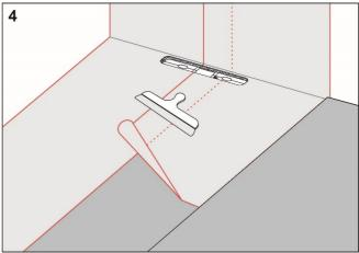
Fit KD+ Folie Trygg or Folie Projekt and overlap the drain collar by a minimum of 50 mm. Seal all seams with KD+ 2K Folielim.
