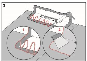
Apply FF M-1K Lim on the drain collar and FF M-1 Membran or FF M-2K to the rest of the floor and wall area.
