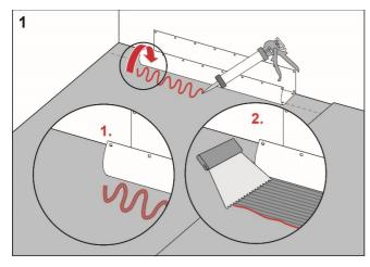
Apply FF M-1K Lim or FF M-2K to the floor and wall areas which the drain collar will cover. Spread the adhesive with a fine-toothed adhesive spreader.
