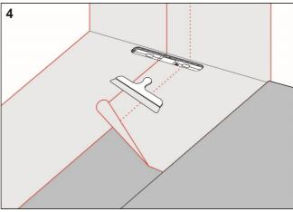
Install FF Folie and overlap the drain collar by a minimum of 50 mm. Seal all seams with FF M-1 Membran, FF M-1K Lim or FF M-2K.
