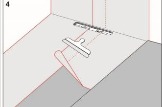
Install Casco Foil and overlap the drain collar by a minimum of 50 mm. Seal all seams with Casco Wetstop iFIX.
