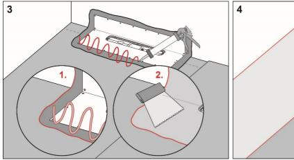
Apply Casco Wetstop Foil Seal to the drain collar and Casco Wetstop iFIX to the rest of the floor and wall area.
