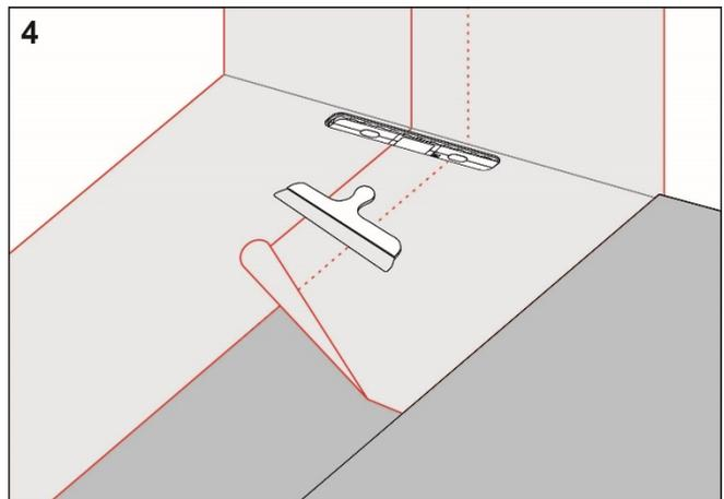
Install Bostik Pro Folie and overlap the drain collar by a minimum of 50 mm. Seal all seams with Bostik Membran, Foil Tac 1C or Foil Seal Cement.
