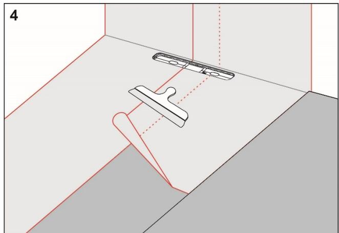
Install Alfix Våtrumsmatta Pro and overlap the drain collar by a minimum of 50 mm. Seal all seams with Alfix 2K Tätningsmassa.
