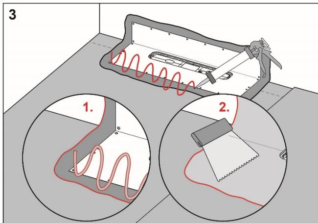
Apply Alfix 2K Tätningsmassa on the drain collar and on the rest of the floor and wall area.
