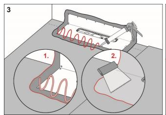
Apply Adda Skarvlim on the drain collar and Adda Membran to the rest of the floor and wall area.
