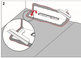
Unfold the collar on the floor and wall. Carefully smooth out the collar and ensure that no wrinkles or blisters occur.
