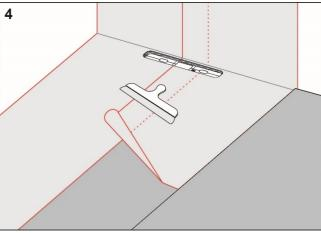
Install Adda Tätfolie and overlap the drain collar by a minimum of 35 mm. Seal all seams with Adda Membran.
