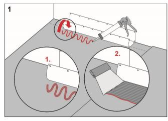
Apply Adda Skarvlim to the floor and wall areas which the drain collar will cover. Spread the adhesive with a fine-toothed adhesive spreader.
