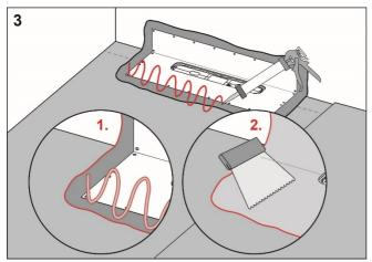
Apply ARDEX 7+8 on the drain collar and to the rest of the floor and wall area. (Use a roller / brush)
