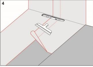
Install ARDEX Foil and overlap the drain collar by a minimum of 50 mm. Seal all seams with ARDEX 7+8.
