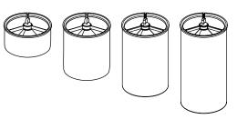
as protection against evaporation, barrier against odour and vermin (two-stage trap effect through water seal and sealing lip membrane)
