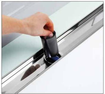
Remove the immersion pipe for cleaning
