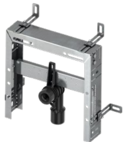
TECEbox washstand module, installation depth 8 cm: To be mounted in front of a solid wall. With four depth-adjustable wall attachments. Installation depth 8-19 cm. Ceramic attachment distance 17-28 cm.
