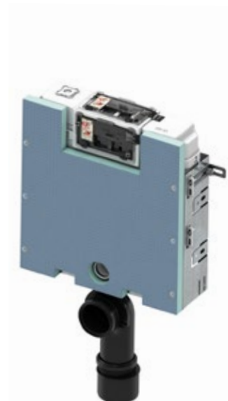
TECEbox toilet module with Uni cistern and tile base front, installation height 820 mm: Toilet module for installation in a bricked-in pre-wall in front of a solid wall, depth-adjustable.
