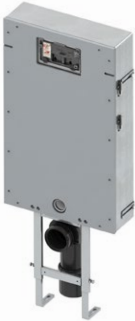
TECEbox toilet module with Uni cistern, with tileable front facing, installation height 1110 mm: Toilet module for installation in a bricked-in pre-wall. Closed surface suitable for tiling made out of glass fibre light concrete. Including pre-assembled height-adjustable supporting feet.
