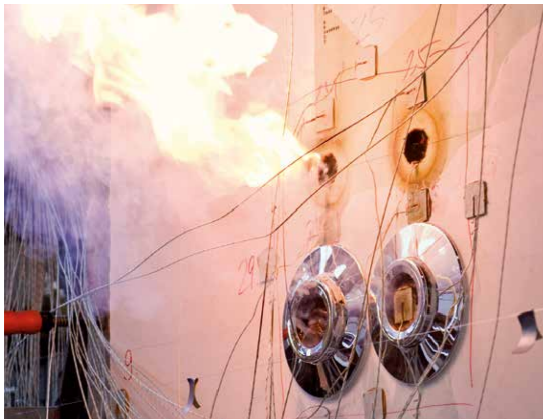
Fire resistance test at the Materials Testing Institute in Braunschweig (Germany). Depending on the design of the bathroom wall section, when exposed to fire on one side, fire resistance classes of up to F 120 were achieved.
