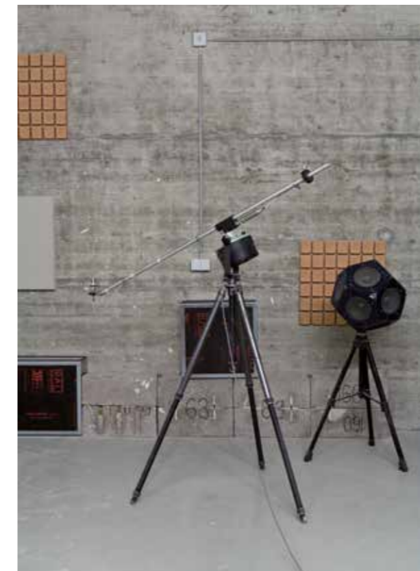
Soundproofing tests on a TECE bathroom wall section at the Fraunhofer Institute for Building Physics. It is wise to have a low level of noise in hotels, but the same is also true for private residences. Special sound-absorbing elements are used in the TECEprofil system to ensure low noise levels. Independent reports confirm the reduced transmission of sound waves in the building structure.
