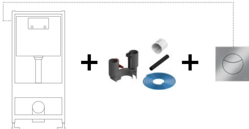
Required components for a pneumatic toilet flush with TECEflushpoint are:
