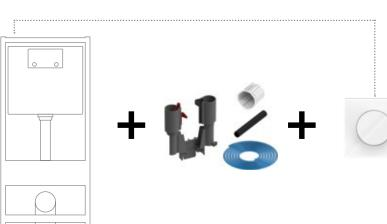
The pneumatic toilet flush with TECEflushpoint always consists of: Toilet module with Octa cistern **TECEflushpoint shell set** for Octa cisterns
