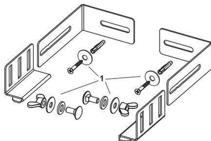
1 668035 Screw set for wall bracket TECEdrainline-Evo
