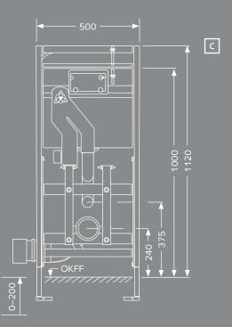
A total of three TECElux modules are available that are each fitted with a dual-flush technology cistern and offer different functions depending on the version, e.g. height adjustment and a ceramic order filter.
