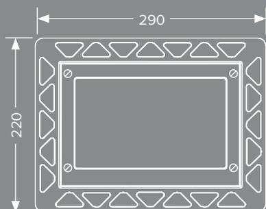
For flush-mounted assembly of TECEnow it's necessary to combine an installation frame and a spacing frame, which both can be ordered separately.
