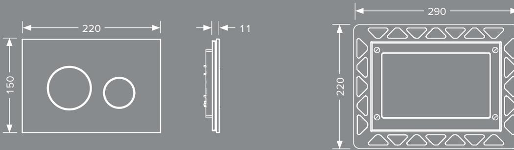
A separate installation frame is available for flush-mounted installation.
