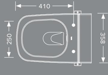
The dimensions of TECEone are especially compact when compared to shower toilets from other manufacturers: The dimensions are comparable to standard toilet ceramics.
