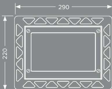
All glass variants offer the unique option of flush-mounted installation thanks to a special installation frame.
