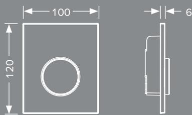
TECEloop flush plate made of plastic including flush valve cartridge for U1 flush valve housing.
