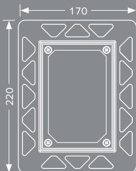
TECEfilo can also be installed flush to the wall in the glass and plastic versions. This requires a special installation frame that is available separately.
