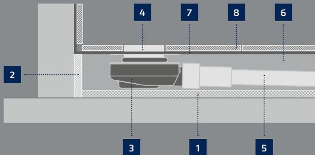
The drain trap is selected according to the drainage capacity required and the available floor installation height. The height for the floor insulation and the drain line gradient should also be considered when making a selection. If the available installation height is insufficient then the shower area can also be designed as a platform with dressing area in the room.
