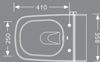
The dimensions of TECEone are especially compact when compared to shower toilets from other manufacturers: The dimensions are comparable to standard toilet ceramics.
