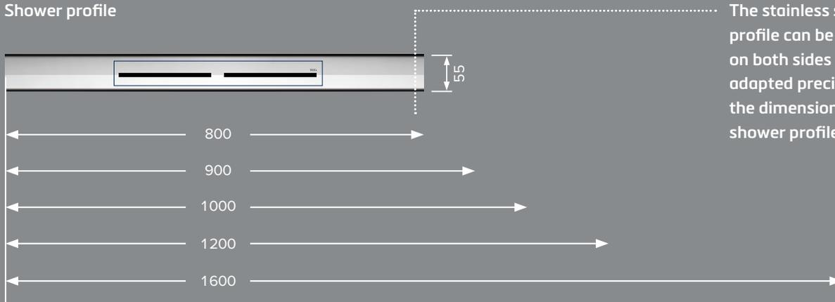
The stainless steel profile can be shortened on both sides and be adapted precisely to the dimensions of the shower profile.
