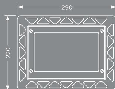
TECEvelvet flush plates can be installed fully flush using a special mounting frame.
