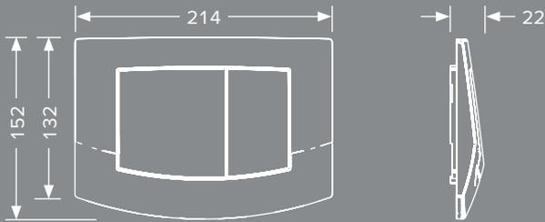
The toilet flush plate made of plastic can be used for front or top actuation. Rattling noises can be reliably avoided during actuations thanks to the rubber buffers on both sides.
