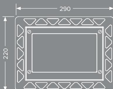
TECElux Mini can also be flush-mounted on the wall with a special installation frame.
