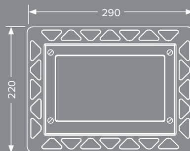
TECESquare flush plates with glass surface can also be installed totally flush using a special mounting frame.
