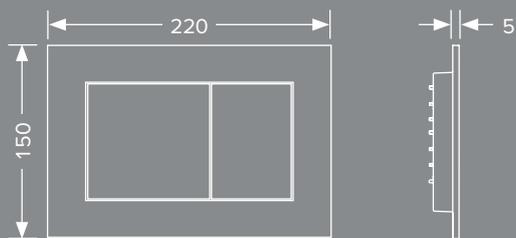
TECEnow is a toilet flush plate made of plastic for TECE cisterns for front or top actuation.
