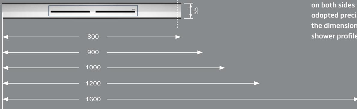
The stainless steel profile can be shortened on both sides and be adapted precisely to the dimensions of the shower profile.
