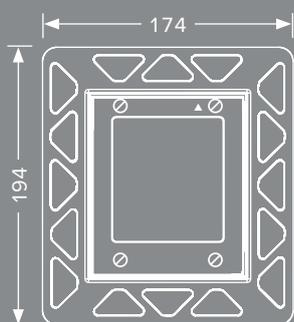
TECESquare can be integrated especially close to the wall (stainless steel) or flush to the wall (glass) via a special installation frame.
