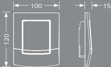
TECEambia urinal flush plate made of plastic including flush valve cartridge for flush valve housing U1.
