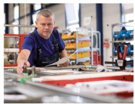
Before shipment, all assemblies are subjected to quality inspection and the multi-stage final inspection. In addition to the completeness of all fixtures, the pipe connections and insulation, we also check the respective accompanying bypack for assembly and connection of the sanitary walls for completeness.
