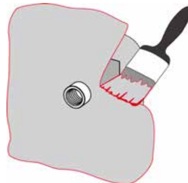
Fig. 3: Applying the upper sealing coating
