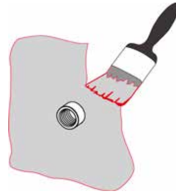
Fig. 1: Applying the lower sealing coating
