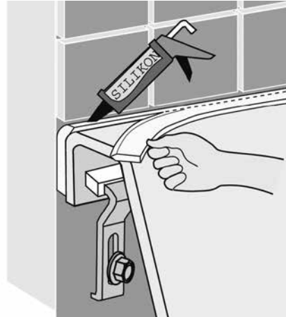
Sealing with bathtub insulation tape and a silicone bead
