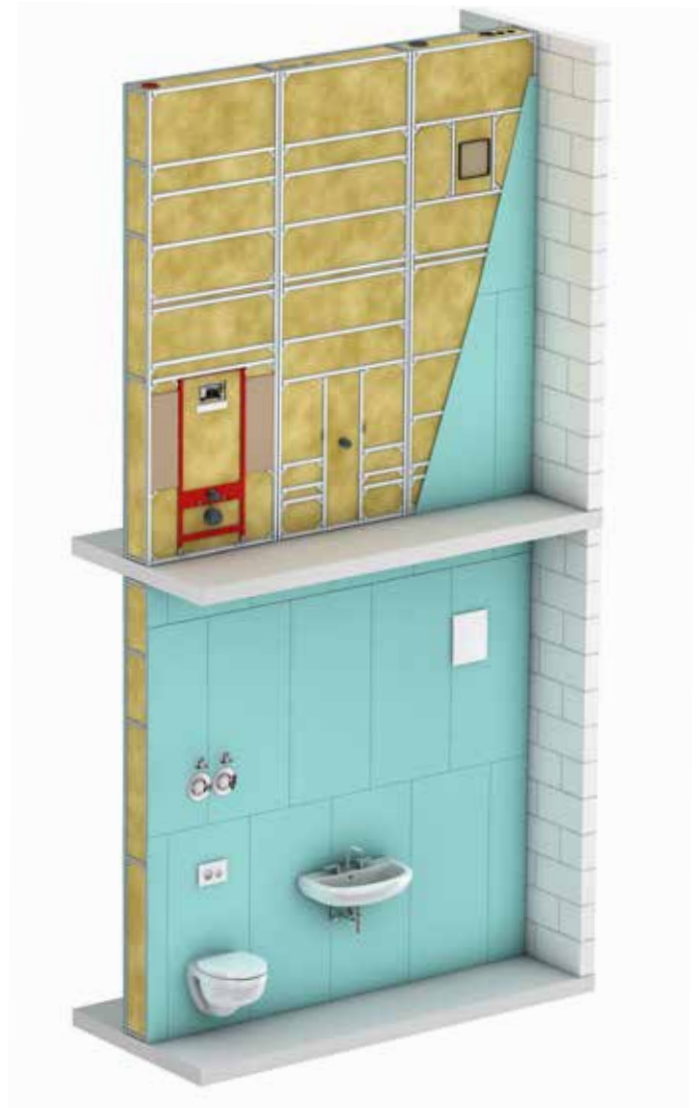
EI 90 from 286 mm wall thickness
