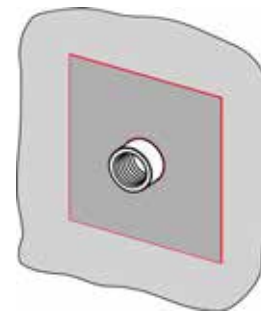
Fig. 2: Bedding the sealing collar into the still-wet sealing coating
