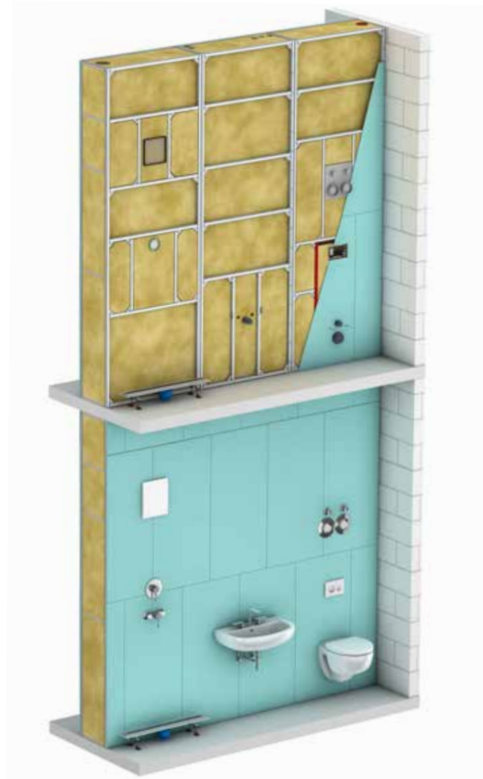
EI 90 from 386 mm wall thickness
