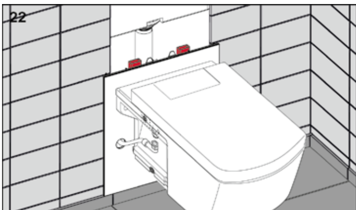
Connect the reinforced hose to the shower toilet.
