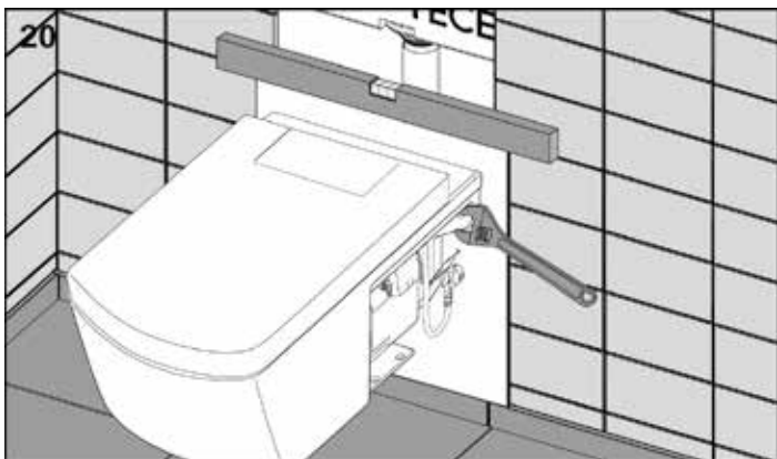
Mount and align the shower toilet.
