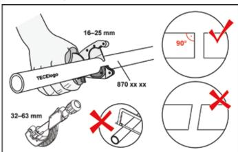
For cutting a TECElogo pipe to length use TECE pipe cutters (order no. 8760002) for the smaller dimensions (up to 25), and use the TECE pipe cutter (order no. 8760008) for the larger dimensions (up to 63)
