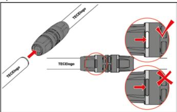
Check the fitting for dirt and clean or swap if necessary. To avoid dirt, do not remove the hygiene caps of the fitting until immediately before the push-fitting operation. Simply push the TECElogo pipe into the fitting until it reaches the stop.
