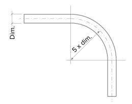
$^{\ast}$  without bending spring; 4 x dim. with bending spring. Minimal bending radius of TECElogo composite pipes
