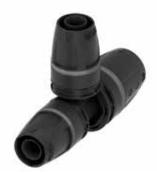
The fitting made of high-performance plastic PPSU is corrosion-free and impact-resistant. It is equally suitable for drinking water installations to DIN 1988/DIN EN 806 and heating installations.
