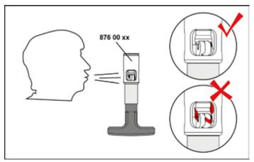
The TECElogo calibrator must be dirt-free. Clean the calibration and chamfering tool after every calibration ("free blowing"). Residual shavings could otherwise be transferred into the sealing zone on the connector.
