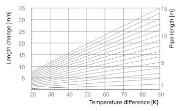
Thermal length extension for TECElogo composite pipes
