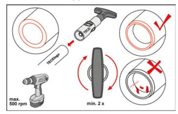
Place the calibration and chamfering tool matching the pipe dimensions (order no. 87600xx) on the end of a TECElogo pipe and turn clockwise multiple times.
