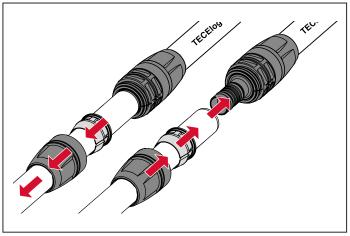
Now push back the collet and clamping ring and pull the pipe away from the fitting base body, then remove the clamping ring and collet from the pipe.
