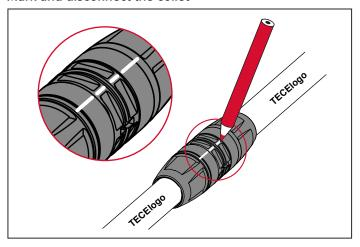
Before undoing a connection, make a continuous marking on the collet and threaded clip. Fix the fitting with the disassembly open-end wrench and unscrew the collet with the dismounting key.
