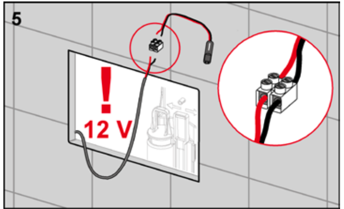
Connect the cable coming out of the transformer to the mains connection adapter (ensure correct polarity – see details in fig. 5).
