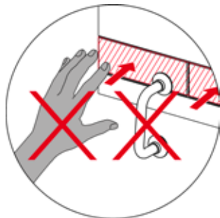
The installed cover can be removed from the flush plate using the bow-type handles included in the installation frame's scope of supply.
