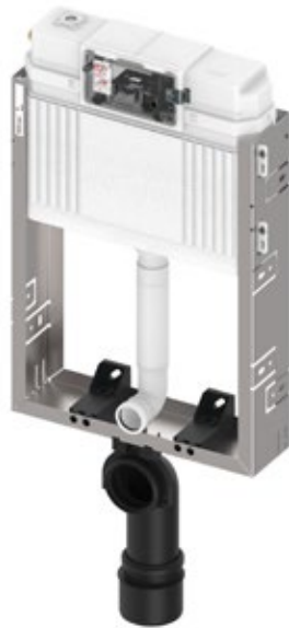
TECEbox toilet module with Uni cistern, installation height 1060 mm: Toilet module for installation in a bricked-in pre-wall in front of a solid wall. Attached in front of or behind solid walls via opposed attachment tabs.
