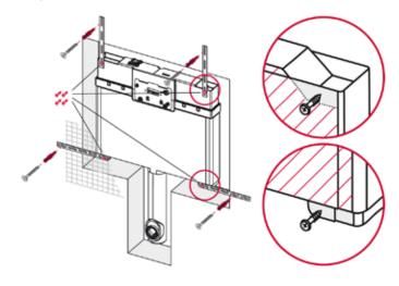
Attach the water connection (connection R 1/2" on the cistern) and then assemble both the polystyrene bare-wall protection and the drainage cover. Brick the module in completely. Fill all cavities and attach the metal mesh.
