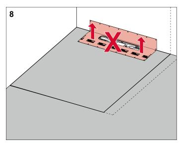
After the sealing sleeve has clicked into place, it may no longer be removed or pulled out again. Otherwise there is a risk that the sealing sleeve could become damaged and that leaks could develop.
