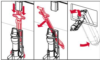
After removing the drainage valve, the valve seat can be removed by pulling it upwards.
