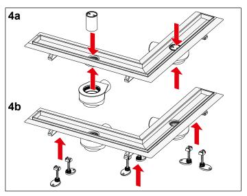
Install the drain and immersion pipe, if necessary clip on the assembly feet.
