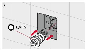
Screw in the mechanical cartridge.
