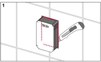
Cut the thin surface of the bare-wall protection with a cutter knife.
