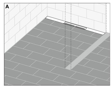
Flush-to-wall position of the drain profile after final installation.
