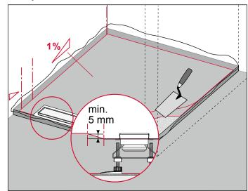
Designing the incline when installing the channel in the middle of the room
