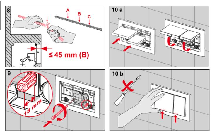
Break off the actuating rods according to the wall structure Finally, replace the buttons manually. and screw them in – distance from front edge of support frame = 18 mm.
