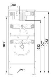
TECEfilo urinal electronics with module (U 2 flush valve housing) 1120 mm
