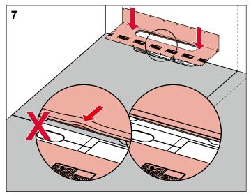
Remove the Seal System sealing sleeve from its packaging and press the frame manually into the slot. The sleeve is correctly installed when it is lying completely flat.
