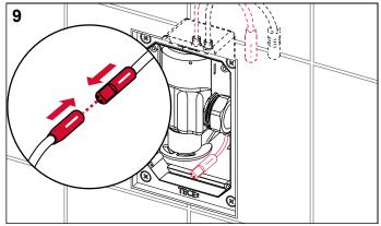
Connect the transformer's plug-in connection.
