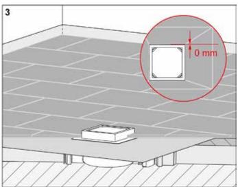
Mount the floor covering without any distance between the bare-wall protection.
