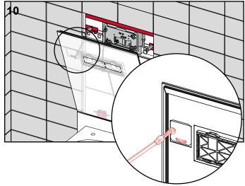
Attach the glass facing with backup tape (hook the snap hook into the eyelet).
