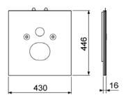
incl. sound insulation kit, and long reinforced pipe. Dimensions:  $430 \times 445 \times 16 \text{ mm}$
