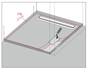
Designing the incline for channel installations "close to the wall"
