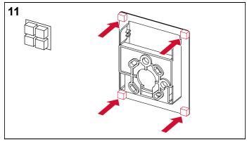
Stick the spacers onto the back of the TECEnow support frame.
