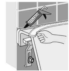
Sealing with bathtub insulation tape and a silicone bead
