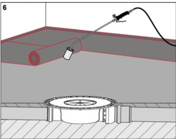
Apply sealing strips (bitumen/EPDM) in accordance with the manufacturer's instructions.
