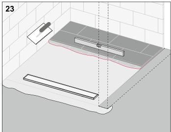
Apply tile adhesive and tiles or natural stone. Observe the necessary 1% incline to the channel.
