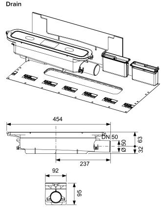
Drain for TECEdrainprofile shower profile, for installing in screed
