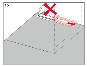
Completely remove the protective sheet from the channel flange. Do not touch the flange any more or let it get dirty.
