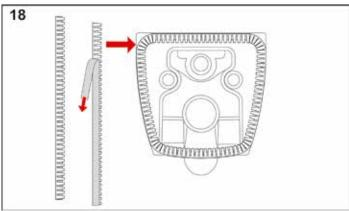
Mount the sound insulation strips on the ceramic.
