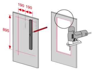
Cutting out the wall recess
