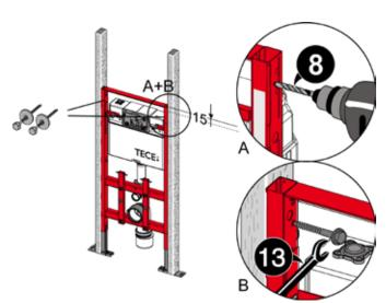
Module attachment during installation in a wooden stud wall
