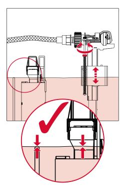
The height should be set so that the water reaches the upper mark on the overflow of the drain valve and the top mark in the cistern (see diagram).
