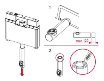
Place the module in the niche, make sure it is level and attach it using perforated rails as shown in the following diagram.
