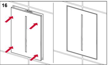
Press the cover into the mounting support.
