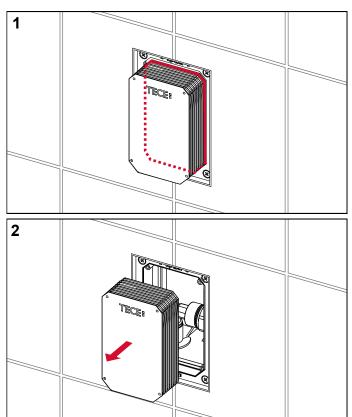
To facilitate installation, we recommend shortening the bare-wall protection to the correct size already when mounting the flush-mounted installation frame. If this has not already been done, shorten the bare-wall protection.
