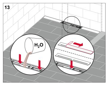
Fill up both odour traps with water. Remove the profile cover, pull off the protective sheet and position the cover.
