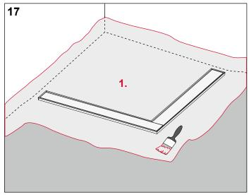
Apply the first coat of composite seal spotlessly over the entire area. In doing so, fully integrate the Seal System sealing tape.
