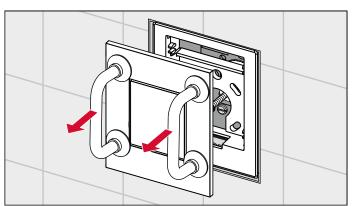
When mounting or dismounting the cover, do not press the button. The installed cover can be removed from the flush plate using the bow-type handles included in the installation frame's scope of supply. Only position the suction cups on the cover to be removed.
