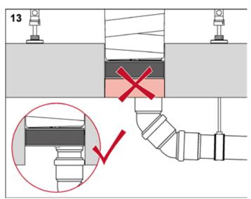
Important: The drilled hole under the fire protection sleeve must not be filled.
