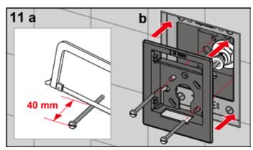
Screw the support frame onto the urinal flush valve housing. If necessary, shorten the two screws so that they do not knock against the mounting cross beam (minimum length on minimum wall structure = 40 mm).
