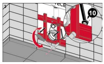
Remove the attachment nuts (x 4) on the depth adjustment, securing the threaded rods at the back in the process.
