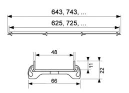
Dimensions of "plate" tileable channel
