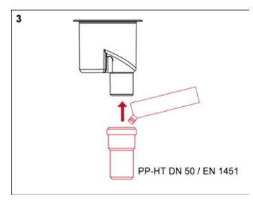
To connect the drain to the wastewater pipe, in the immediate area around the fire protection sleeve, use a PP-HT pipe DN 50 with a wall thickness of 2 mm (according to DIN EN 1451-1: 1999).
