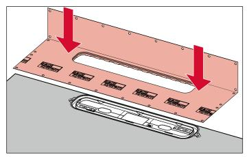
The flexible sealing sleeve must then simply be integrated into the composite seal.
