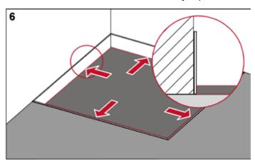
The sound-proofing mat should cover the whole floor surface.
