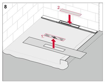
Place the protective cover over the shower profile opening so that nothing can get into the drain during the further course of the construction work.
