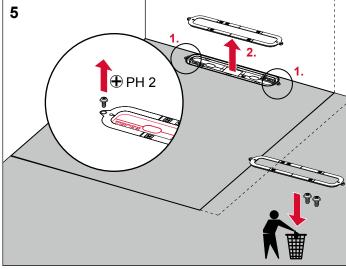
Loosen both screws and remove the external part of the protective cap.
