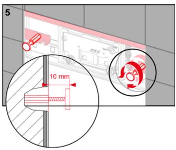
Screw in both magnetic holders – 10 mm in front of the wall surface.
