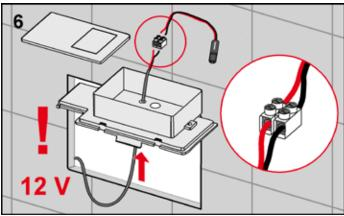
Open the cistern cover and remove it with the installation box. Guide the (12 V) transformer cable from beneath through the opening in the bottom of the box and connect it to the mains connection adapter (ensure correct polarity – see details in fig. 6).
