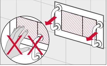
When mounting or dismounting the cover, do not press the button; the cover should only be removed using the suction handles.
