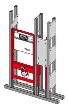
Installing the module for safety support arms and support systems in a free-standing wall with a flush-mounted profile
