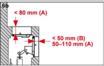
Break off the actuating rods according to the thickness of the wall structure.
