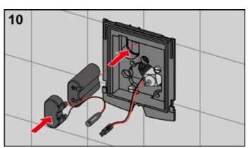
Place the connector adapter on the battery and position it in the opening provided for the purpose.
