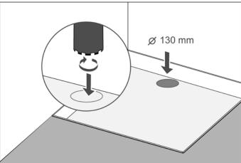
Drill a core hole with Ø 130 mm.
