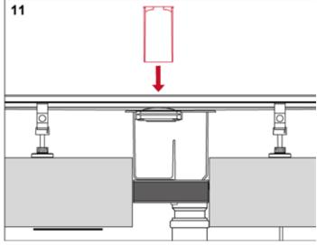
Insert the immersion pipe into the channel body.
