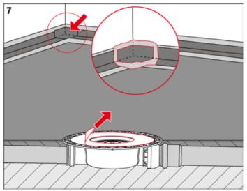
Attach corner seal(s), remove protective film from flange.
