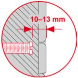
Screw in both attachment rods – distance of attachment rod to wall surface: 10 - 13 mm.
