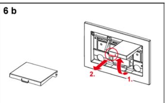
Manually dismount both buttons from the flush plate by bending up the snap-in hooks towards the button. To avoid damaging the buttons, do not use a screwdriver or similar tool.
