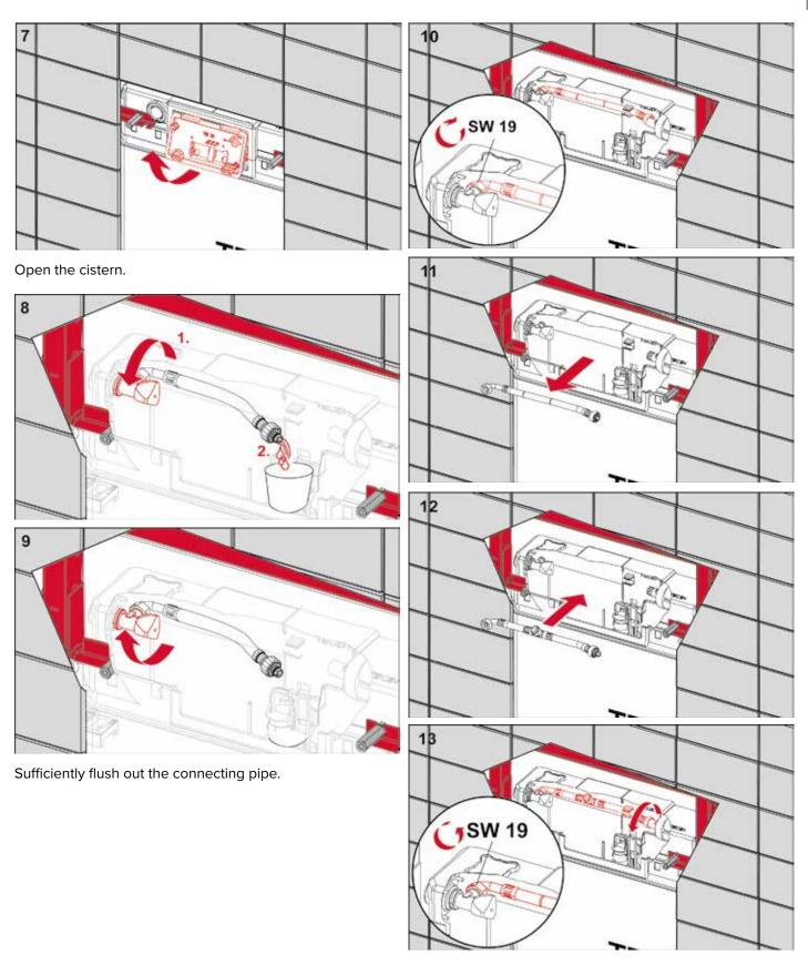
Remove the reinforced hose and replace it with the replacement reinforced hose with the water connection for the shower toilet or shower toilet seats.
