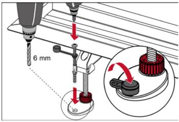
After alignment, the feet can be secured in the floor through the Drainbase sound-proofing mat. Then press the sound insulation caps onto the bolt heads. This will prevent a sound bridge from forming.
