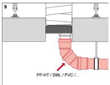
Transitions to other commercially available types of pipe and materials (made of PP-HT, SML, PVC, etc.) can be connected to the first PP-HT pipe.
