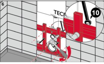
Then secure the threaded rods at the back and tighten the locking nuts.
