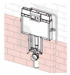
Fill all cavities and attach the metal mesh (see diagram).
