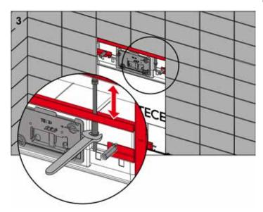
On TECElux modules 200 and 400, it is possible to lower the height 20 mm downwards or raise it 60 mm upwards – compared with the module frame's factory settings.
