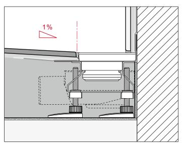
Insert the channel cover. Lay the cover flush with the floor in the shower channel.
