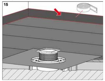
Apply the edge insulation strips.
