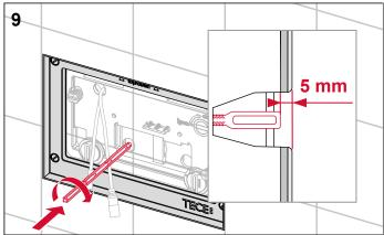
Screw in both actuating rods – distance of actuating rods to wall surface = 5 mm.
