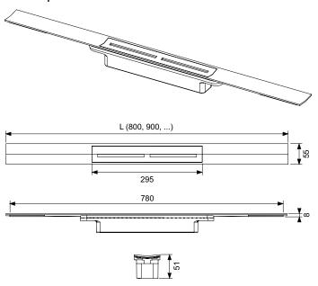
Shower profile for shower drainage, for installation in the tile adhesive above the screed and seal.
