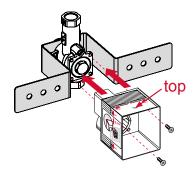
The bare-wall protection housing is cut flush to the wall after tiling.
