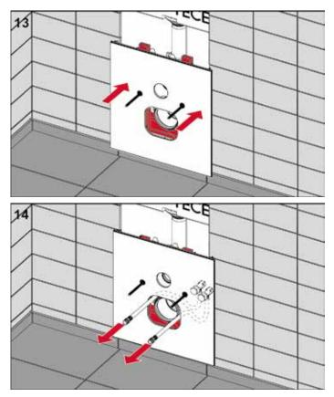
Mount the glass facing and guide the reinforced hose through the large opening on the glass facing to the front.
