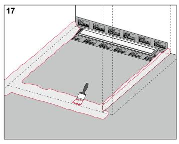
Apply a coat of composite seal to the transitions between the wall and the screed. Observe the manufacturer's instructions when creating the composite seal (figs. 17 to 23).
