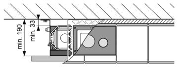
"Flush-mounted installation from above" - minimum wall structure
