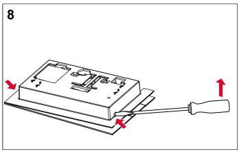
Remove the cover from the flush plate using a screwdriver. Place the screwdriver into the recesses on the underside of the flush plate and carefully remove the cover.
