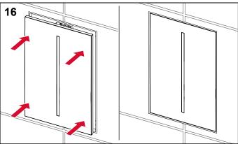
Press the cover into the mounting support.
