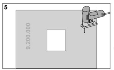
Saw the required opening for the installation frame in the board.
