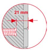
Screw in both attachment rods – distance of attachment rods to wall surface = 21 mm.
