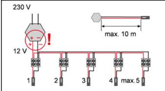
Connect the transformer cable to the mains connection adapter. Ensure correct polarity when making the connections.
