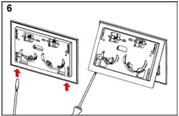
The cover and flush unit are supplied ready-mounted, and must be separated for the installation. Remove the cover from the flush plate using a screwdriver. Place the screwdriver into the recesses on the underside of the flush plate and carefully remove the cover.
