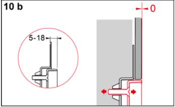
Adjust the depth of the installation frame to the tile thickness (5–18 mm). If the wall structure is thicker (up to 33 mm), as is the case for example with natural stone, you can use a suitable upgrade kit (order no. 9820181).
