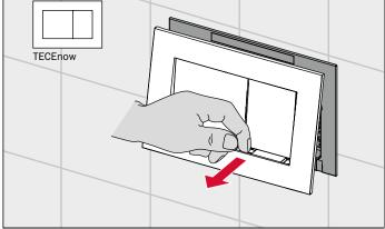
The flush plate cover for the TECEnow can be removed by hand. For the TECEsquare II, use the bow-handles.
