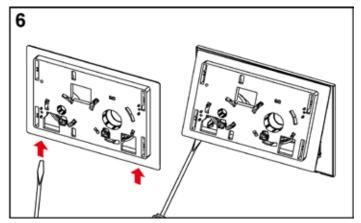
The cover and flush unit are supplied ready-mounted, and must be separated for the installation. Remove the cover from the flush plate using a screwdriver. Place the screwdriver into the recesses on the underside of the flush plate and carefully remove the cover.
