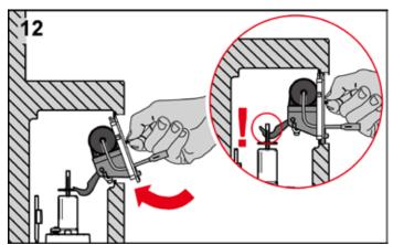
Insert the splash guard for the electronics with the actuation motor. The activation hooks must fit correctly in the drain valve's drawbar eyelets. Tighten the splash guard clamping screws.
