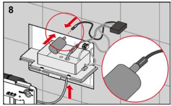
Connect the electronics first to the motor (black plug) and then to the batteries (grey plug). If the installation is correct, the motor will be activated once for checking purposes.
