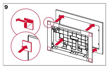
Push the distance frame onto the support frame and stick the spacers onto the support frame.
