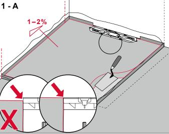
The drain must be inserted into the screed in such a way that it fits flush with the top surface of the screed.
