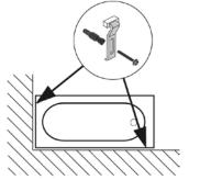
Securing the bathtub using bathtub anchors
