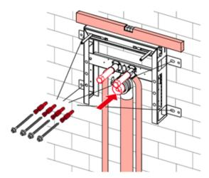
With the washstand module, you must set the distance between the threaded rods (minimum value 170 mm, maximum value 280 mm).
