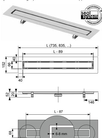
Straight channel body and support sheet for TECEdrainline shower channel, for installation in the screed and onsite laying of large tiles/natural stone slabs, with flange and Seal System\* sealing tape, for creating a tested and certified connection of the TECEdrainline channel to the composite seal.
