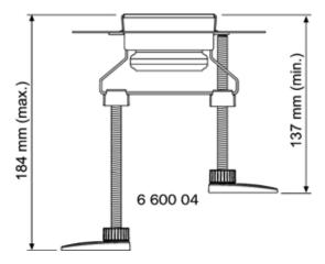
The adjustment range from the lower edge of the feet to the upper edge of the finished floor for item number 660004 is 137-184 mm. When the "Max" drain is installed, these longer mounting feet must be used.
