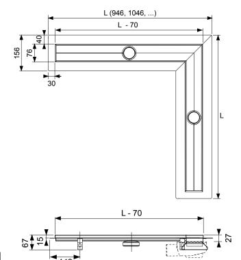
Shower channel with 90° angle for installation in the screed, with flange and Seal System\* sealing tape for creating a tested and certified connection of the TECEdrainline channel to the composite seal.
