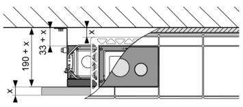
"Flush-mounted installation from above" - wall structure (suggestion)
