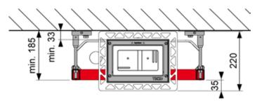
"Flush-mounted installation from above" - dimensions
