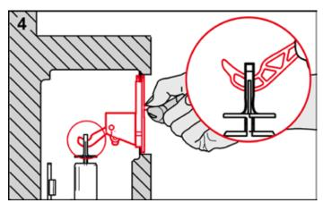
The activation hooks must fit correctly in the drain valve's drawbar eyelets. Tighten the splash guard clamping screws.
