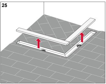
Remove the protective cover, clean the channel.
