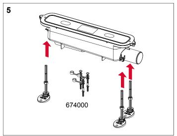
Manually screw in the assembly feet at the drain.
