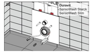
Mount the Duravit electronic connection box (following the Duravit installation instructions) or V & B connector plug (following the V & B installation instructions).
