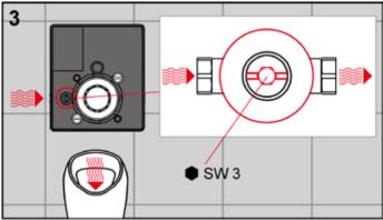
Sufficiently flush out the pipe.
