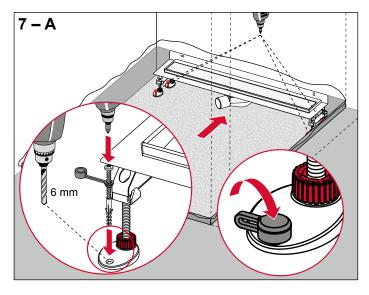
Place the channel at the wall. Either attach the assembly feet as shown here, and press the sound insulation caps on to the bolt heads, or ...
