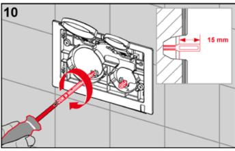
Screw in the actuating rods through the corner supports – distance to front edge of support frame = 15 mm.
