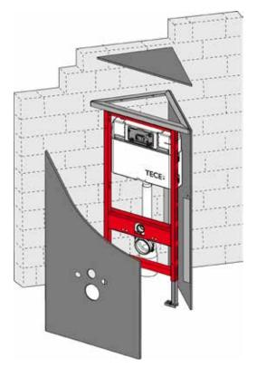
Mounting the module attachment for wall corner installation
