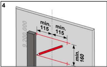
Mark the dimensions of the inside of the installation frame – width 230 mm, height 160 mm – in the centre of the plasterboard.
