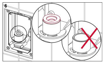
Make sure that the connection piece is fitted with a seal. This seal can be greased if necessary.
