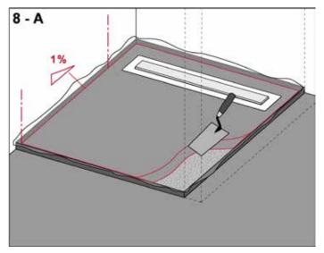
Use the adjustable assembly feet to raise the shower channel to the required position and align horizontally, if necessary, pack the drain body.
