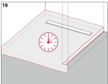
Spotlessly complete the first coat of composite seal.
