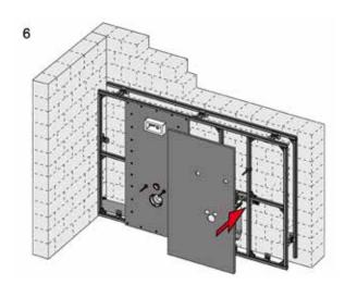
Make the cut-outs in the panel plates, put the facing in place
