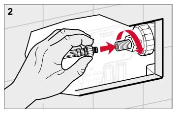
Turn the corner valve to close it again and connect the reinforced hose to the filling valve. If you wish to fill the cistern with water (e.g. for the initial operation), you must open the corner valve again.
