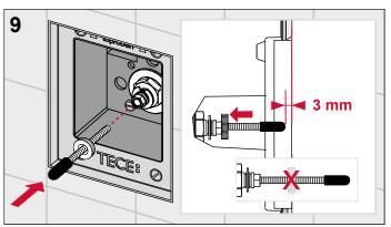
Screw in the actuating rods as described above (for flush-mounted TECEsquare, distance to front edge of inside of installation frame = 3 mm), and screw on the counter nut to prevent them from turning.
