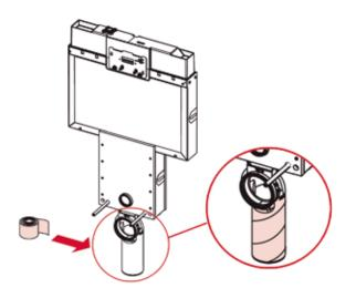
Place the module in the nice and attach the water connection (connection R 1/2" on the cistern).
