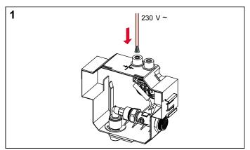
The transformer is already integrated into the flush valve housing to facilitate coordination of the different trades carrying out the assembly work. Therefore, the transformer can be directly connected with a 230 V cable.
