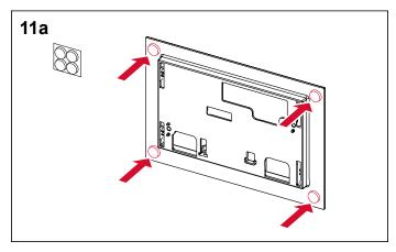
Stick the spacers onto the back of the TECElux Mini's support frame.
