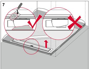
Pack the drain body if it is not lying flat. Remove the protective cover and push in the immersion pipe up to the stop.
