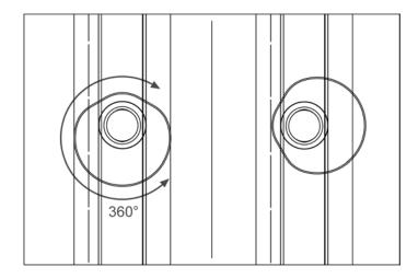
When the installation is close to the wall, the body of the drain body can be turned. In this case, there is no need to chisel into the wall.
