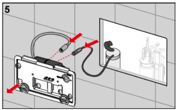
Guide the cable for the actuation motor and battery through the opening in the splash guard so that it is easier to connect in the next step.
