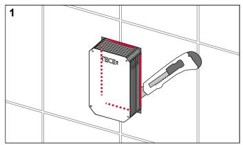
Cut the thin surface with a cutter knife.
