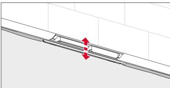
The shower profile is finely positioned by installing the drain in screed. The assembly solution allows subsequent fine positioning of the shower profile in all horizontal directions.
