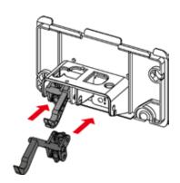
When replacing an old A1 drain valve with a new A2 one, care must be taken to ensure that the operating lever is also replaced.
