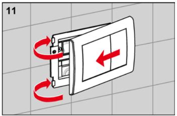
Hook the cover of the TECEambia flush plate into the righthand side, and fit it onto the support frame by means of the snap lock.
