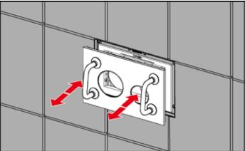
Remove the support frame and polystyrene bare-wall protection. Then mount the matching support frame as described in the respective installation instructions (TECE-loop or TECEsquare). Finally, insert the flush plate into the flush-mounted installation frame with the aid of the bow-type handles. The handles are included in the installation frame's scope of supply.
