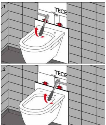
The height can then be adjusted via the adjusting screw. For "quick adjustment", the ceramic can also be raised slightly. Find adjustment is then carried out using the adjusting screw.
