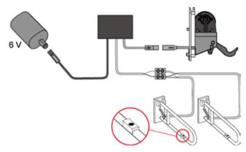
When the electric circuit to the switch on the safety support arm is closed, the flush is activated. In addition to the electrical supply, the switch on the safety support arm and the actuation motor, an additional electronic component must also be installed between the different components. Power is supplied by a 6 V battery.
