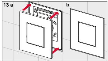
Allow the cover of the TECEnow flush plate to click into place in the support frame.
