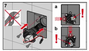
Install the electric cartridge (do not insert with tool!) and tighten the screws by hand.
