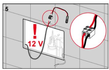
Connect the cable from the transformer to the mains connection adapter (ensure correct polarity – see details in fig. 5).
