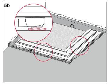
If necessary pack the drain body.
