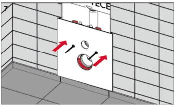
Mount the lower glass facing with actuation unit and — if not already carried out at the factory — insert both glass protection caps.
