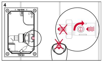
Before mounting the flusher, make sure that the inlet flow control is closed so that no water can leak out during assembly. Close the shut-off using a flat-head screwdriver. In the free-flow setting (fig. 3), the shut-off slot is parallel with the housing, and in the closed setting (fig. 4), it is at right angles to the housing.
