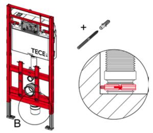
Vertical installation of the flexible drain bend (TECElux 200 and 400)
