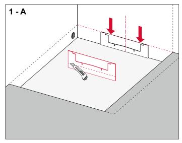
Before applying the screed, the special sound insulation strips supplied must be shortened to the required height. This should be shortened in such way that the top surface of the sound insulation strip fits flush with the surface of the screed.
