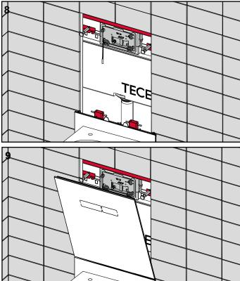
Insert the upper flush plate into the supports and lift up.
