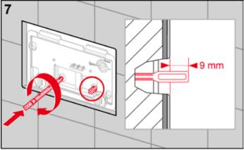
Screw in both actuating rods – distance of actuating rods to wall surface = 9 mm.
