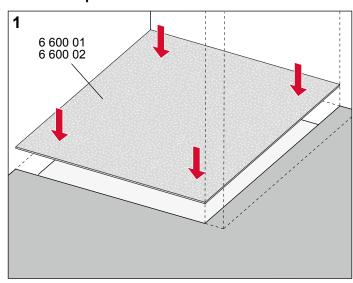
Optional: Cut the drainline sound-proofing mat and place in position so that it covers the whole surface of the shower area.
