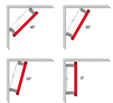
Installation examples with module attachments for variable corner installations
