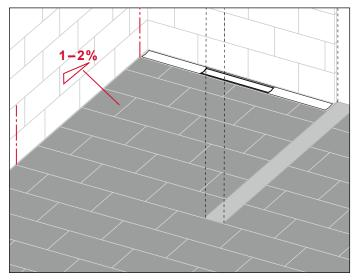
"Flush-to-wall" installation, incline
