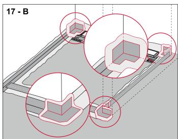
Apply the composite seal to the corners and fold and fit the corner seals, making sure that there are no air bubbles.
