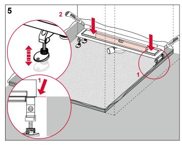
Use the adjustable assembly feet to raise the channel to the required height and align horizontally, if necessary pack the drain body.
