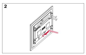
Insert the anti-theft device into the glass cover mounting supports.
