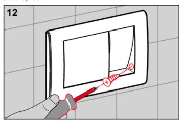
Then screw the vandal-resistant screw into the inside of the flush plate (caution: be careful not to damage the surface).
