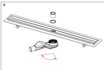
Place the drain on the channel body.
