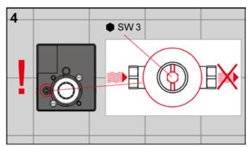
Before mounting the cartridge, ensure that the inlet flow control is closed so that no water can leak out during assembly. Close the shut-off using an Allen key. In the free-flow setting (fig. 3), the shut-off slot is parallel with the flush valve housing and in the closed setting (fig. 4), it is at right angles to the housing.
