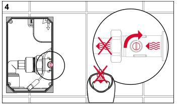
Before mounting the flusher, make sure that the inlet flow control is closed so that no water can leak out during assembly. Close the shut-off using a flat-head screwdriver. In the free-flow setting (fig. 3), the shut-off slot is parallel with the housing, and in the closed setting (fig. 4), it is at right angles to the housing.
