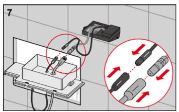
Connect the radio electronics first to the motor (black plug) and then also to the batteries (grey plug). If the installation is correct, the motor will be activated once for checking purposes.
