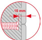
Screw in both attachment rods – distance of the rods to wall surface = 10 mm.
