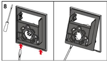
Loosen the support frame from the cover by inserting a screwdriver into the notches on the underside.
