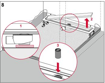
Completely pack the drain body. Remove the protective cover sheet and insert the immersion pipe.
