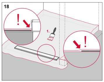
Apply the first coat of composite seal spotlessly over the entire area. When doing so, fully integrate the Seal System sealing tape.
