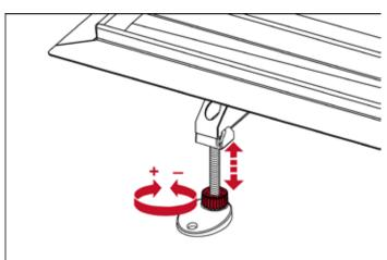
The height of the channel is set by turning the red adjusters on the feet. Check the alignment of the shower channel using a spirit level.
