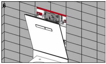
Insert the upper flush plate into the supports.
