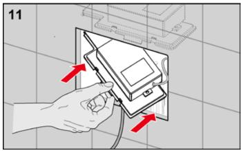
Place the electronics and the battery in the installation box, seal and place back in the cistern.
