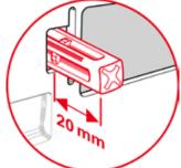
Screw in the actuating rods – distance to front edge of support frame = 20 mm.
