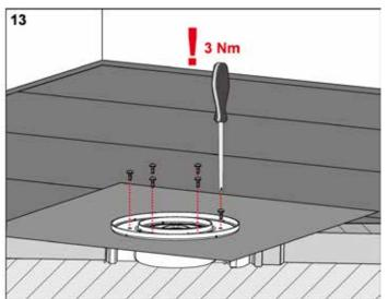
Screw on the compression ring (torque 3 Nm!).
