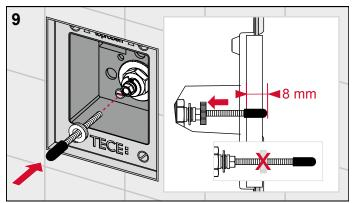
Screw in the actuating rods as described above (for flush-mounted TECEnow, distance to front edge of inside of installation frame = 8 mm), and screw on the counter nut to prevent them from turning.
