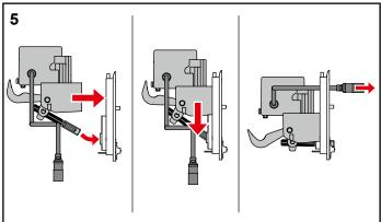
Push the actuation motor onto the splash guard.
