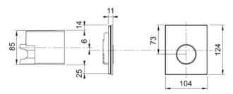
Urinal flush plate and bare-wall protection for vertical slot alignment
