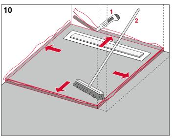
Cut off any protruding edge insulation strips and PE sheet, clean the screed.
