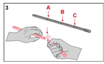
Cut the actuating rod to a suitable length.
