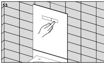
Carry out a function test on the flushing system or program the electronics.
