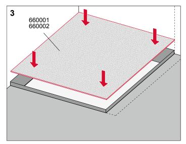
Introduce the Drainbase sound insulation mat, cutting it down to size beforehand if necessary. Here too, you must make sure that there are no gaps or holes in the screed to prevent sound bridges from forming between the screed and the uncovered floor.
