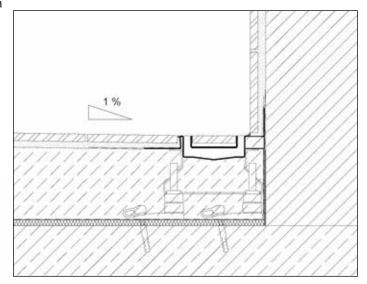
Installation "directly at the wall", incline
