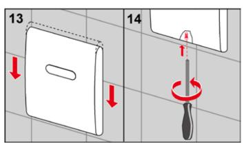
Finally, install the flush plate cover and mount the vandal-resistant screw supplied.
