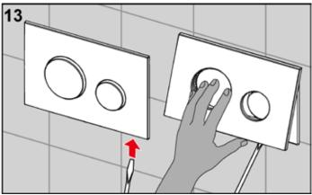
The installed cover can be detached from the flush plate using a screwdriver. To do this, insert the tool into the recesses on the underside of the flush plate and carefully remove it.
