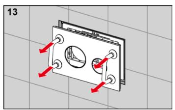
The installed cover can be removed from the flush plate using the bow-type handles included in the installation frame's scope of supply. Only position the suction cups on the cover to be removed.
