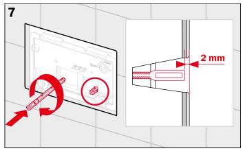
Screw in both actuating rods – distance of actuating rods to wall surface = 2 mm.
