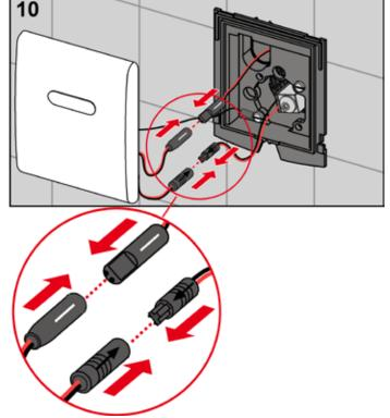
Connect the battery and cartridge to the electronics.
