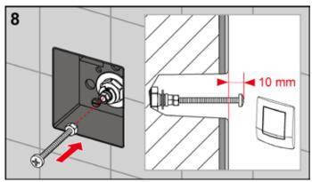
Screw in the actuating rods as described above (for the TECEambia, distance to wall surface = 10 mm) and screw on the counter nut to prevent them from turning.
