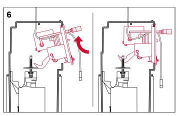
Place the splash guard and actuation motor back in the cistern.
