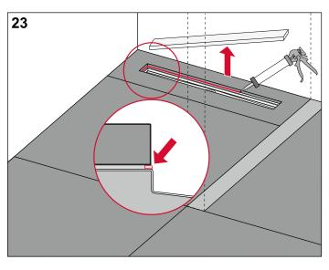
Seal the space between the floor covering and the screed with permanently flexible material.
