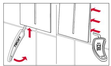
To dismount the cover, insert the programming key into the notches on the underside of the flush plate.
