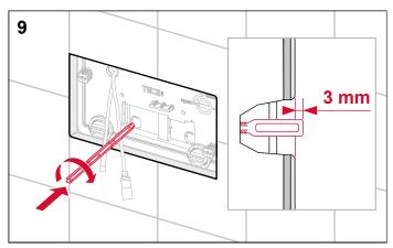
Screw in both actuating rods – distance of actuating rods to wall surface = 3 mm.
