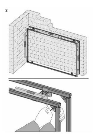
Use a spirit level to align the section tube and connect using corner joints
