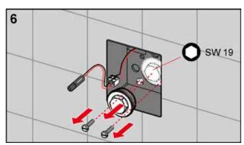
Remove the bare-wall plug and unscrew the fastening screws on the bare-wall protection.
