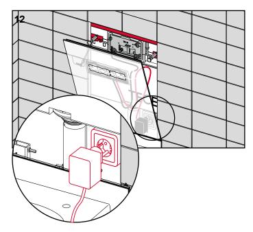
Plug the plug-in power pack into the socket.
