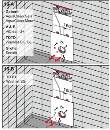
Guide the reinforced hose and power cable through the sewage water connection or side opening in the glass attachment facing.
