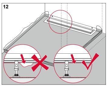
Make sure that there are no cavities between the screed and the channel or drain.
