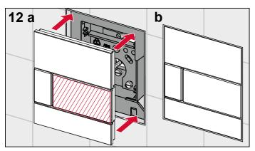
Allow the TECEsquare flush plate cover to click into place in the support frame.
