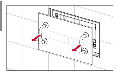
The installed cover can be removed from the flush plate using the bow-type handles included in the installation frame's scope of supply.
