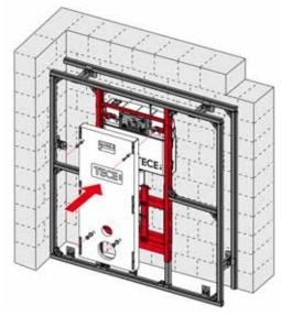
Attach the bare-wall protection to the module.
