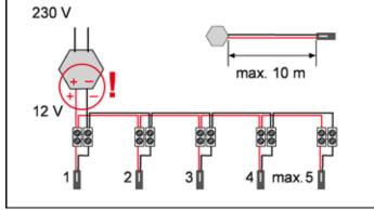
Schematic diagram of a series installation of 5 urinal electronic units
