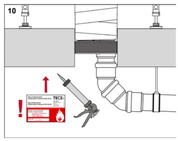
Attach a completed identification plate in a clearly visible and permanent manner – e.g. with silicone – next to the pipe closure system beneath the ceiling.
