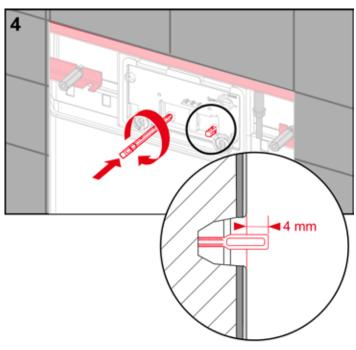
Screw in the actuating rods -4 mm in front of the wall surface.
