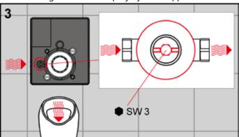
Sufficiently flush out the pipe.
