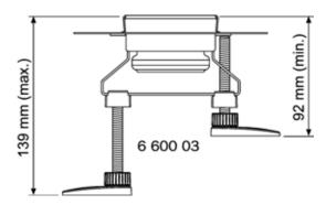
The adjustment range from the lower edge of the feet to the upper edge of the finished floor for item number 660003 is 92–139 mm.
