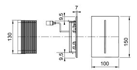
Dimensions of glass urinal electronics and bare-wall protection for vertical slot alignment
