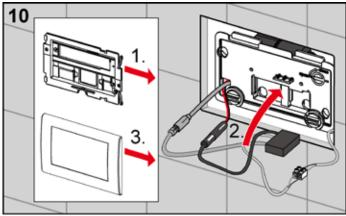
Mount the flush plate support frame and install the electronics in a suitable location (e.g. between the support frame and the flush plate). Finally, install the flush plate.
