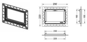
Flush-mounted installation frame for toilet flush plate
