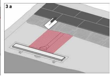
Due to the partially limited screed covering, a sufficiently wide piece of reinforcement fabric must be worked into the area between the drain and the outlet pipe.
