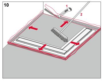
Apply screed with the necessary incline – in the shower zone – of at least one percent to both channels. The reverse gradient should be at least 5 mm.
