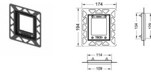
Flush-mounted installation frame for urinal flush plate
