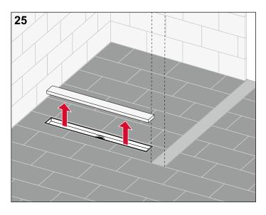
Remove the protective cover and clean the channel.
