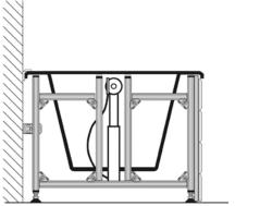
TECEprofil supporting frame when installing an overflow fitting
