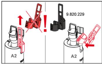
On cisterns installed after mid/end of 2009 and which contain the drain valve (A2) shown, the valve's red pull rod must be replaced by a black one. This is supplied with the toilet electronics motor or is available as a replacement part (order no. 9820229).
