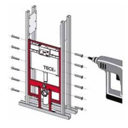
Attach the water connection (connection 1/2" FI on the cistern) and clad the wall with plasterboards. Ensure that openings are left for the flush plate, drainage and threaded rods. The total thickness of the coating (board, adhesive and tiles) must be at least 18 mm.
