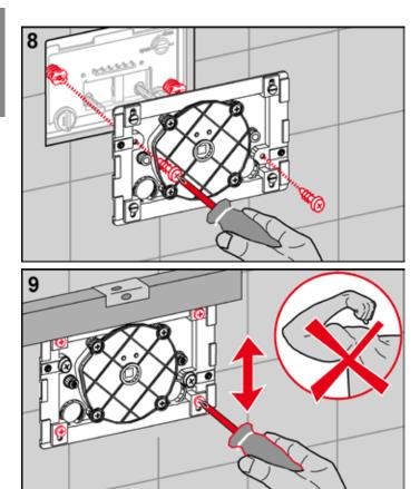
Screw the rotary mechanism onto the attaching rods and align them horizontally.
