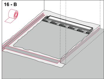
Apply a coat of composite seal to the transitions between the wall and the screed. Observe manufacturer's instructions when creating the composite seal (figs. 15-A to 22).
