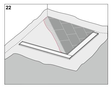
Apply the floor covering (tiles, etc.), allowing for the specified incline in the process.
