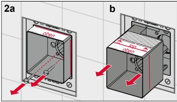
First, mark the bare-wall protection protrusion, and remove the polystyrene support. Loosen the screws and remove the bare-wall protection.
