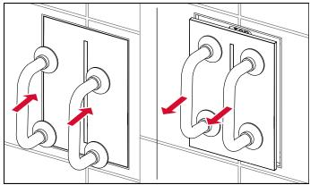
The installed cover can be removed from the flush plate using the bow-type handles included in the installation frame's scope of supply. Only position the suction cups on the cover to be removed.
