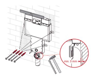
Attach the water connection (connection R 1/2" on cistern). Brick the module in completely and follow the outline. Install the polystyrene bare-wall protection, the threaded rods and the odour traps.
