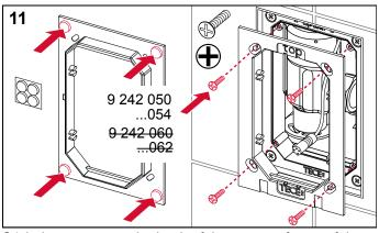
Stick the spacers to the back of the support frame of the plastic electronics, and screw the frame onto the urinal flush valve housing.
