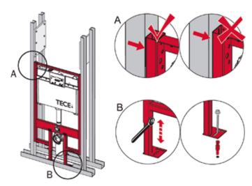
Attach the sides of the module to the supports on the frame.
