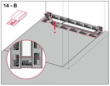
Cut the Seal System sealing tape to length, remove the protective film and fold the tape, overlapping it over the channel flange and screed as illustrated, then stick it down, pressing with a roller and making sure that there are no air bubbles.
