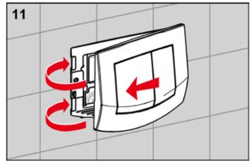
Hook the cover of the TECEambia flush plate into the righthand side, and fit it onto the support frame by means of the snap lock.
