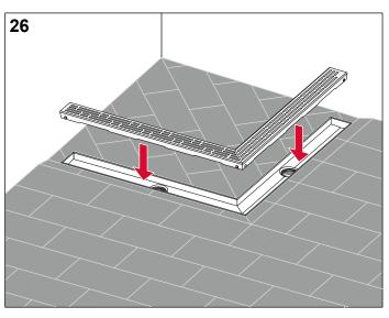
Insert the required cover (design grate, tileable channel).
