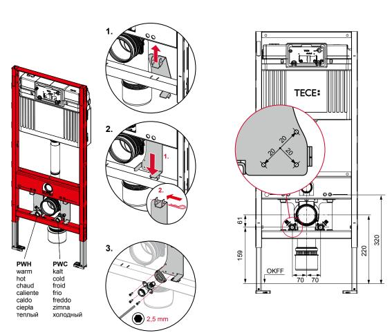
A short stub line from the circulating hot water pipe to the module is recommended for the TECEone's hot water connection. This ensures that, when the water is circulating, hot water will come out of the shower rod immediately after the water supply has been opened. With a longer hot water stub line, by slightly opening the water inlet, cooled water will flow into the ceramic.
