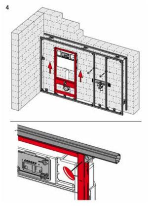
Pull out the module, secure it to the top section tube with corner joints, apply the foot brake and close the clip on the module foot
