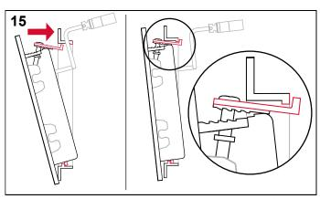
The top of the anti-theft device must be detached for the installation.
