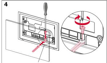
Attach the anti-theft device to the support frame with the screw supplied.
