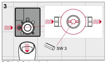
Sufficiently flush out the pipe.
