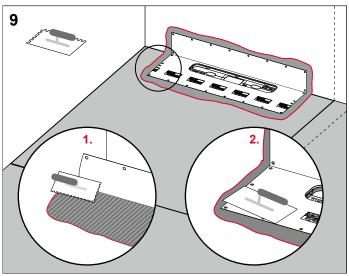
Install the sealing sleeve evenly across the whole area of the liquid-applied sealing material and press it down.
