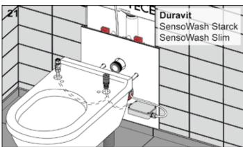
Guide the power and water connections through the ceramic according to the Duravit or V & B installation instructions.
