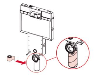
Remove the rear sound insulation plate.
