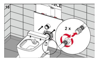
Connect the reinforced hoses to the TECEone connection hoses.
