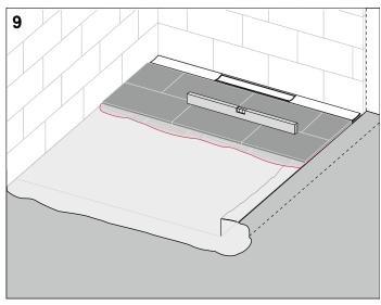
Lay the floor covering (8-25 mm including adhesive bed) with the required incline (1–2 %) towards the shower profile.
