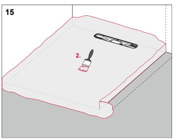
After the first coat has dried, apply the second coat over the entire surface.
