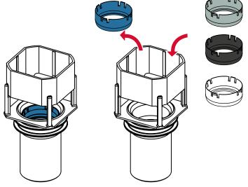
The flush flow throttle can be easily installed in the valve seat of the drainage valve.
