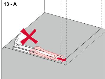
Completely remove the protective sheet from the channel flange. Do not touch the flange any more or let it get dirty.
