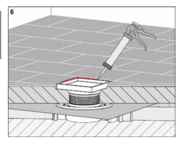
Seal the joint with permanently flexible material.
