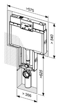
Place the module in the niche and attach the water connection (connection R 1/2" on cistern). Install the polystyrene bare-wall protection, the threaded rods and the odour traps. Make sure the module is level and brick it in completely. Fill all cavities as you do this.
