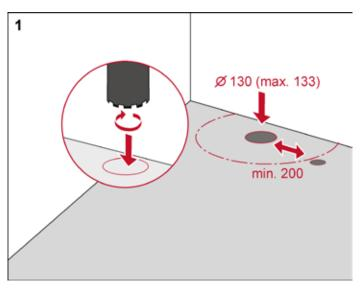
Make a core hole for the drain, diameter 130 mm (max. 133 mm). The distance to the nearest ceiling duct must be at least 200 mm.
