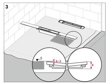
As is the case for every floor drainage element, the shower profile is the deepest element installed in the shower zone. Therefore it should be installed at the same height, or slightly deeper, than the subsequent tiles.
