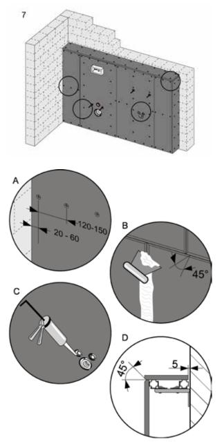
Covering the TECEprofil supporting frame with facing, and filling
