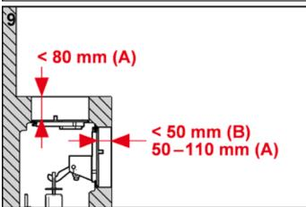
Break off the attachment rods according to the wall structure.
