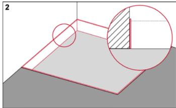
Apply the edge insulation strips along the wall and to the existing screed surfaces.
