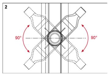
The turning range of the extra-flat drain is approx. 90° to either side of the shower channel.
