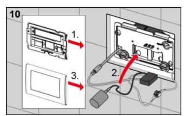
Mount the flush plate support frame and install the electronics and the batteries in a suitable location (e.g. between the support frame and the flush plate). Finally, install the flush plate.
