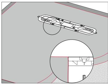
The shower profile can be cut to size and easily and precisely adjusted to fit the width of the shower area. This is carried out by means of a hand saw with a stainless steel hacksaw blade.
