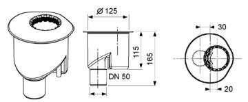
Vertical drain for TECEdrainline shower channel to create rotatable fitting with the channel body and side connection to DN 50 wastewater pipe, with removable siphon immersion pipe
