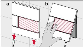
To dismount the cover, insert a screwdriver into the notches on the underside of the flush plate.
