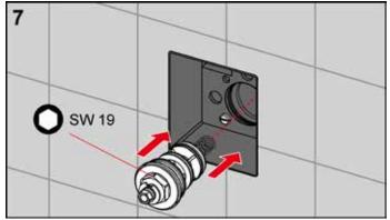
Screw in the mechanical cartridge.
