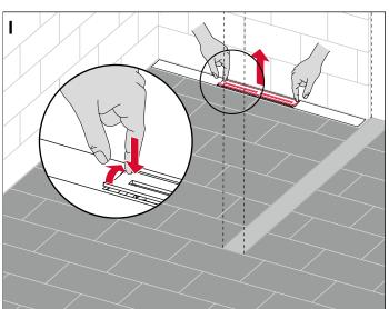
To do so, press the rear edge of the profile cover downwards. Doing this will slightly tile the cover upwards; then it can be lifted up by hand.
