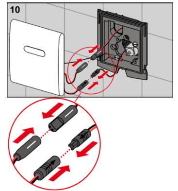
Connect the electronics to the mains and to the cartridge.
