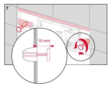
Screw in both magnetic holders – 10 mm in front of the wall surface.
