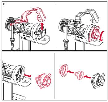
If necessary, you can obtain replacement parts for the filling valve with order numbers 9820382 (valve lever set) and 9820383 (sealing kit).
