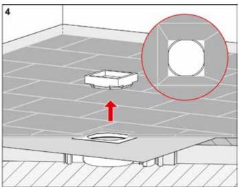
Remove the bare-wall protection.
