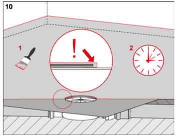
Apply second sealing coating over complete area: The sealing sleeve must be completely covered by the damp-proof coating. Allow coating to dry.
