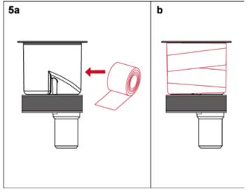
Place a spiral duct, or wrap adhesive binding or other sound insulation material around the drain body - **not the sleeve**.
