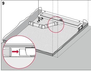
Attach the wastewater pipe to the outlet socket.
