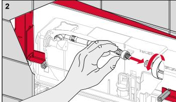
Sufficiently flush out the connecting pipe and screw on to the filler valve.
