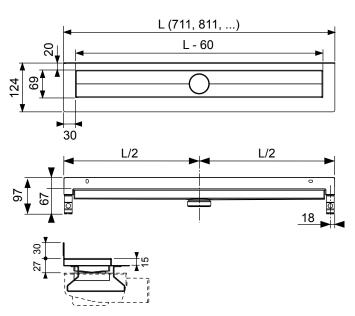
Straight shower channel with wall upstand for installation in the screed against the wall, with flange and Seal System\* sealing tape, for creating a tested and certified connection of the TECEdrainline channel to the composite seal.
