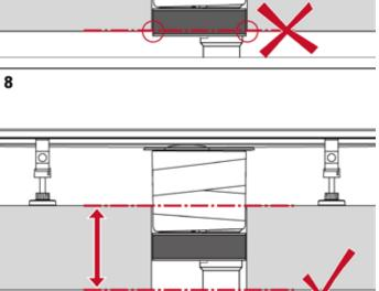
The fire protection sleeve should not protrude above or below the concrete ceiling.
