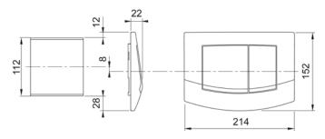
Dimensions of toilet flush plate and bare-wall protection for vertical slot alignment
