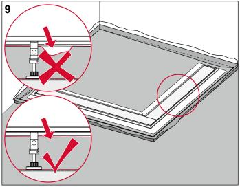
Remove the protective cover, check for leaks and replace the protective cover.
