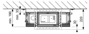
"Flush-mounted installation from above" - dimensions
