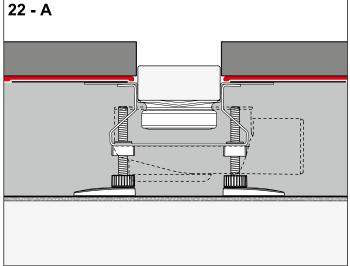
Installation close to the wall (A): Lay the floor covering in the remaining shower area with the required incline of at least one percent to the shower channel.
