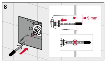
Screw in the actuating rods as described above (for the wall-mounted TECEsquare, distance to front edge of inside of installation frame = 9 mm) and screw on the counter nut to prevent them from turning.
