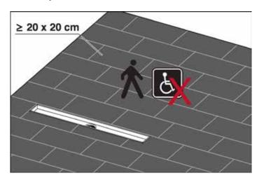
When choosing the floor covering, it should be taken into account that only slabs with an edge length of at least 20 cm should be used. The shower area is not suitable for wheelchairs.
