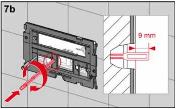
Break off the actuating rods according to the thickness of the wall structure. Screw in both actuating rods – distance to front edge of support frame = 9 mm.
