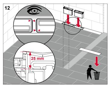
Remove the protective cover and insert both odour traps. When doing so, the arrows on the odour trap and supports should lie directly opposite each other. Then push in the odour trap up to the stop. If necessary, the push-in depth can be checked by measuring (25 mm from the top edge of the odour trap to the top edge of the profile opening).
