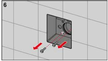
Unscrew the fastening screws on the bare-wall protection.
