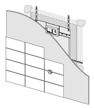
The wall construction must be at least 18 mm if the actuation is located on the wall (A). A minimum of 30 mm is required to install the TECEsquare II (B) and when using the flush-mounted installation frame (C).
