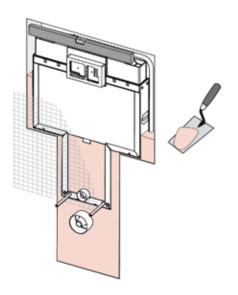
Attach the metal mesh, then plaster and tile the wall.
