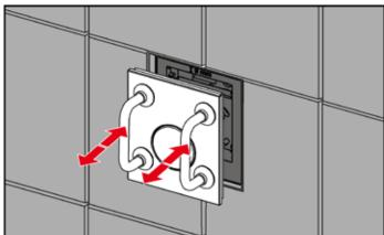
Remove the support frame and proceed as described in the installation instructions (installing the urinal cartridge, installing the support frame, etc.). Finally, insert the flush plate into the flush-mounted installation frame with the aid of the bow-type handles. The handles are included in the installation frame's scope of supply.
