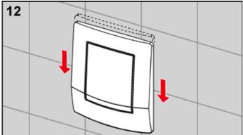
Finally, mount the flush plate cover (here, TECEambia).
