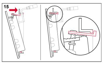
The top of the anti-theft device must be detached for the installation.
