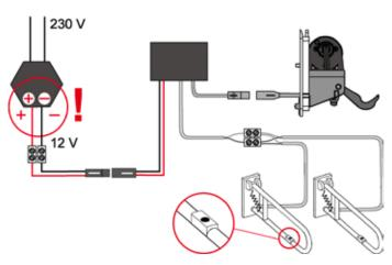
When the electric circuit to the switch on the safety support arm is closed, the flush is activated. In addition to the electrical supply, the switch on the safety support arm and the actuation motor, an additional electronic component must also be installed between the different components. To connect the 12 V mains variant, the power supply must be transformed to 12 V DC by a TECE transformer (order transformer separately: order no. 9810003).
