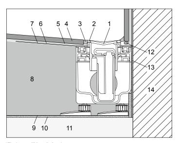
"Flush-to-wall" installation, layer structure:
