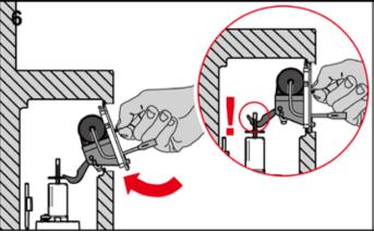
Guide the actuation motor cable through the opening in the splash guard.
