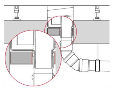
As temperatures rise during a fire, this material foams up to many times its original form.
