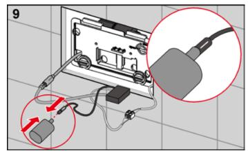
Then, connect the electronics first to the motor (grey plug) and then also to the batteries (black plug). If the installation is correct, the motor will be activated once for checking purposes.
