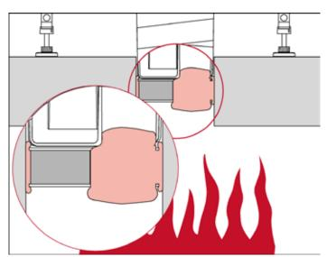
In the socket area, the outflow nozzle including the pushed-on HT pipe sleeve becomes crushed.
