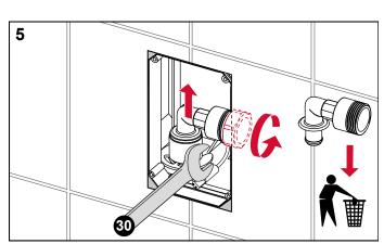
Loosen and remove the flush pipe elbow.
