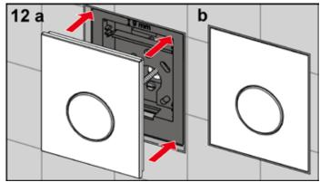
Allow the TECEloop flush plate cover to click into place in the support frame.
