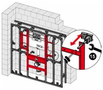
Installation in a TECEprofil pre-wall
