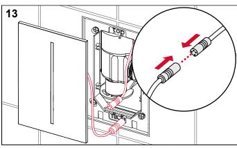
Connect the plug-in connection for the infrared sensor on the cover plate.
