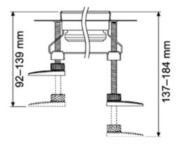
Assembly feet adjustment range: 6 600 03 (left) and 6 600 04 (right)
