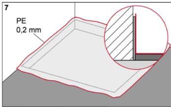
Lay out the PE film as shown.
