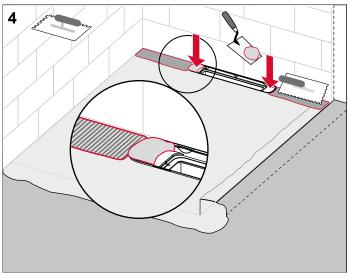
The shower profile is installed with tile adhesive following the "buttering-floating" method. To this end, the tile adhesive is applied to the floor and the deepened elements of the drain. Make sure that no tile adhesive gets into the drain or on the seal.
