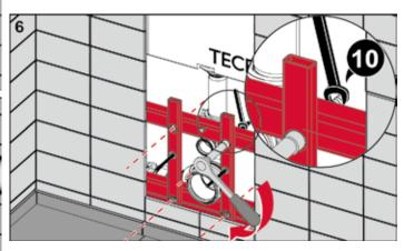
Then secure the threaded rods at the back and tighten the locking nuts.
