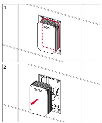
To facilitate installation, we recommend shortening the bare-wall protection to the correct size already when mounting the flush-mounted installation frame. If this has not already been done, shorten the bare-wall protection.
