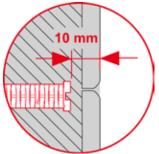
Screw in both attachment rods – distance of attachment rods to wall surface = 10 mm.
