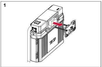
Disassemble the splash guard including the flush unit.
