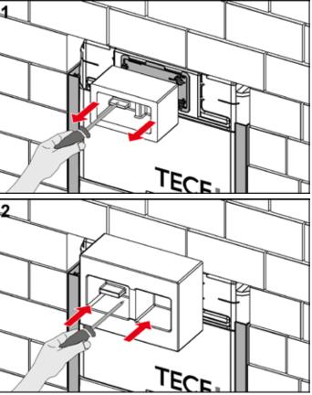
Remove the standard bare-wall protection and mount the larger brick-wall bare-wall protection for flush-mounted installations (order no. 9030029).
