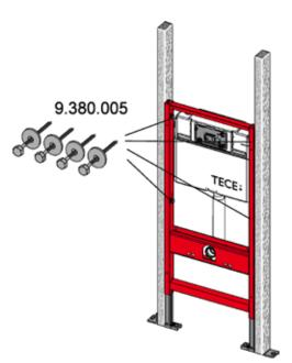
Module attachment during installation in a wooden stud wall
