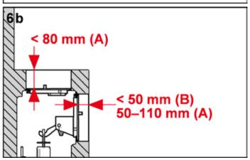
Break off the actuating rods according to the wall structure.
