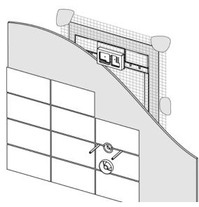
The wall construction must be at least 18 mm if the actuation is located on the wall (A). A minimum of 30 mm is required to install the TECEsquare II (B) and when using the flush-mounted installation frame (C).
