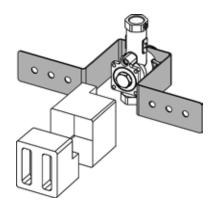
The urinal flush valve housing with TECE valve is already pre-mounted on an attachment plate and can easily be inserted into the slot in the wall. The big advantage of this urinal flush valve housing is its total compatibility with manual or electronic actuation variants. This means the flush plate can be swapped out at any time, even after assembly.
