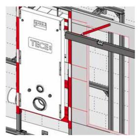
Transfer the markings to the plaster board
