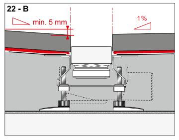
Installation in the middle of the room (B): Lay the floor covering in the remaining shower area with the required incline of at least one percent to the shower channel. The reverse gradient must be at least 5 mm.
