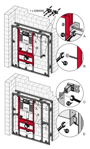
Installation of mounting plates for safety support arms with wall fixing (above) or multi-clips and section tube (below)  $\,$
