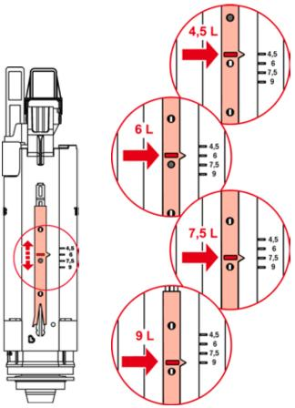
A2 drain valve, adjusting the flush volume
