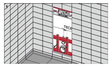
Remove the bare-wall protection.
