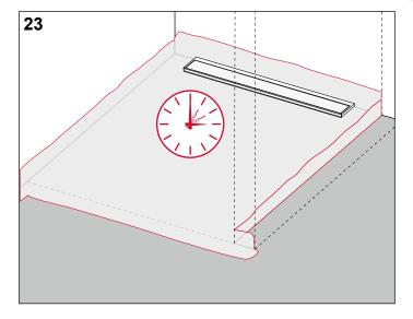
Allow the composite seal to harden, observe the specified drying time.
