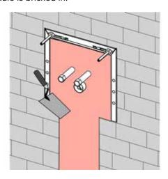
The plaster is then applied and the surface can be tiled.
