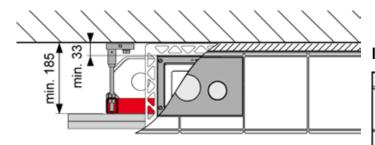
"Flush-mounted top actuation" installation – minimum wall structure
