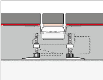
Clean the shower channel, insert the support sheet into it, and check the spacing dimensions.
