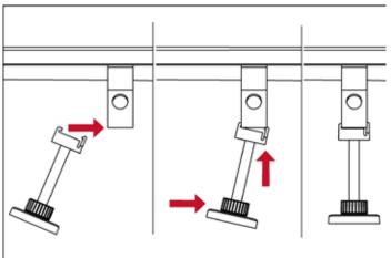
Hook the assembly feet in place, engage the clips and align them.
