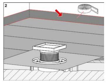
Apply the edge insulation strips.
