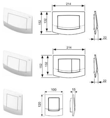
TECEambia toilet flush plate, single-flush technology TECEambia toilet flush plate, dual-flush technology TECEambia urinal flush plate
