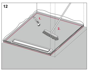
Remove the edge insulation strips and PE sheet above the screed. Clean the screed surface.
