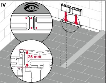
Push in the odour traps up to the stop in the profile supports. When doing so, the arrows on the odour trap and supports should lie directly opposite each other. If necessary, the push-in depth can be checked by measuring (25 mm from the top edge of the odour trap to the top edge of the profile opening). Finally, insert the profile cover again.
