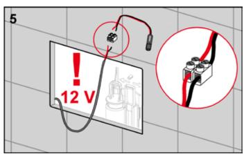
Connect the cable coming out of the transformer to the mains connection adapter (ensure correct polarity – see details in fig. 5).
