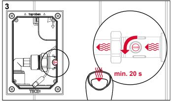
To flush out the connection pipe, open the inlet flow control and sufficiently flush out the pipe.
