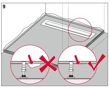
Make sure that there are no cavities between the screed and the channel or drain.
