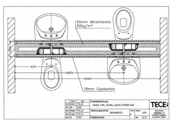
Construction of the tested TECEprofil dividing wall
