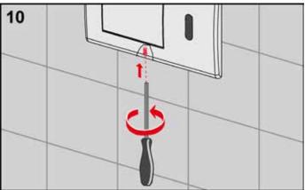
Hook the cover of the TECEplanus flush plate into the right-hand side and fit it onto the support frame by means of the snap lock. Then screw the vandal-resistant screw from underneath into the flush plate (caution: be careful not to damage the surface).
