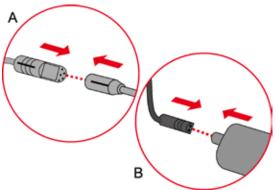
Connect the electronics to the actuation motor and the battery via the plug. If installed correctly, directly after connecting all plugs and the power supply, the electronics will automatically activate the motor once.
