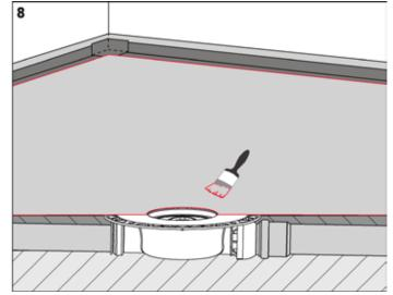
Apply first sealing coating over complete area.
