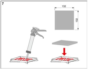
Cut the floor covering (approx.  $132 \times 132 \text{ mm}$ ) and bond in the tileable channel with flexible adhesive (e.g. silicone or epoxy resin adhesive).
