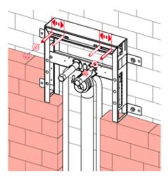
Brick the module in completely and fill all cavities.
