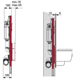
Dimensions of side view and wall construction following detailed installation
