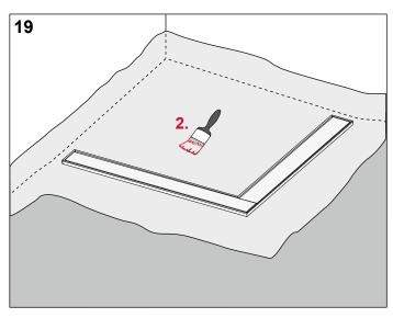
Apply the second coat of composite seal spotlessly over the entire area.
