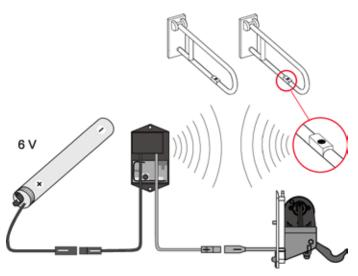
The radio signal sent when the radio switch is activated is received by a radio receiver. This receiving unit operates the power circuit to trigger the actuation motor. Power is supplied via four batteries enclosed in waterproof housing in the cistern.
