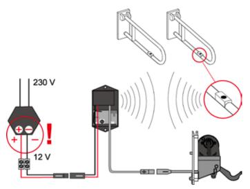
The radio signal sent when the radio switch is activated is received by a radio receiver. This receiving unit operates the power circuit to trigger the actuation motor. To connect the 12 V mains variant, the power supply must be transformed to 12 V DC by a TECE transformer (order transformer separately: order no. 9810003).
