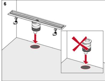
Place the drain on the channel body and move to the required position.
