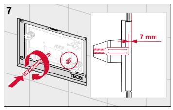
Screw in both actuating rods - distance of actuating rods to wall surface = 7 mm.
