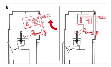
Insert the splash guard with the electrical actuation motor (included in the upper glass facing's scope of delivery of the ). No conversion of drain valve required.
