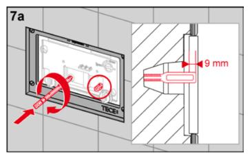
Screw in the actuating rods – distance of actuating rods to front edge of inside frame = 9 mm.
