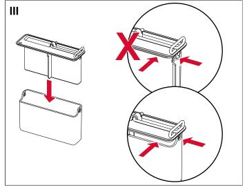
After cleaning, put the odour traps back together.
