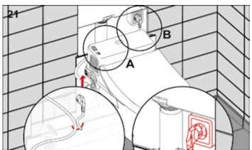
Connect the reinforced hose to the shower toilet seat (A) and connect the power supply: Insert the plug into the socket (B).
