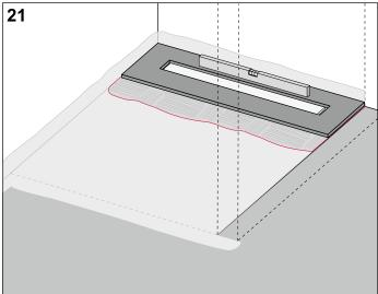
Apply the second coat of composite seal spotlessly over the entire area.
