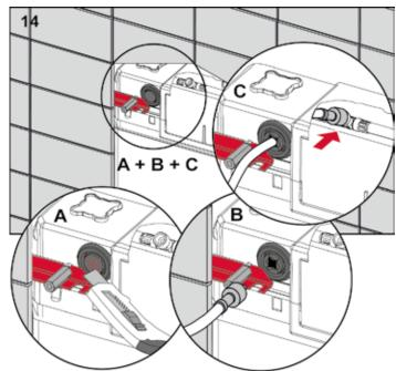
Cut the insertion opening with a cutter knife, insert the reinforced hose into the cistern and connect.
