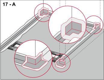
Fold the sealing tape and fit it directly into the connection in the fresh composite seal, making sure that there are no air bubbles.
