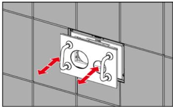
Remove the support frame and polystyrene bare-wall protection. Then mount the matching support frame as described in the respective installation instructions (TECE-loop or TECEsquare). Finally, insert the flush plate with the aid of the bow-type handles (supplied with the installation frame) into the flush-mounted installation frame.
