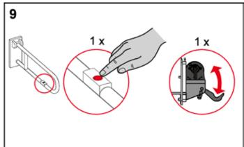
Now check that the function is working: To do this, press the button again to activate the motor (once).
