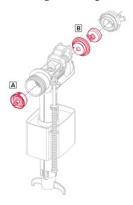
The inlet component (A) or the membrane of the pilot valve (B) can be cleaned if they become dirty due to polluted water.
