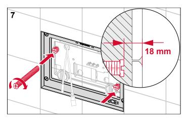
Screw in both attachment rods – distance of attachment rods to wall surface = 18 mm.
