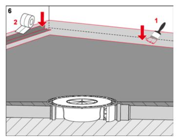
Attach sealing collar and sealing tape in the transition between the screed and the wall (and if necessary to other screed areas).
