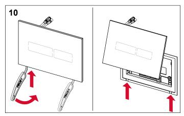
The cover can be detached from the flush plate using the disassembly tool. To do this, insert the tool into the recesses on the underside of the flush plate and carefully remove the cover.
