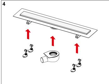
Mount the drain and click on the assembly feet if applicable.
