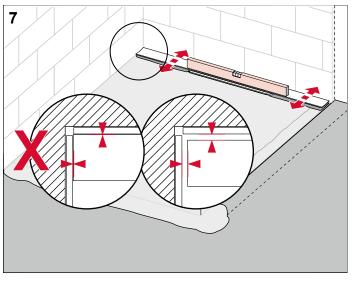
Adjust the height of the profile (also see illustration 3) and align horizontally. When aligning, make sure that the shower profile and wall tiles do not come into contact. The surrounding joint will later be filled in a permanently flexible way with sanitary silicone.
