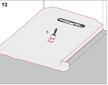
Finally, directly apply the first coat of sealing material weton-wet over the entire surface.
