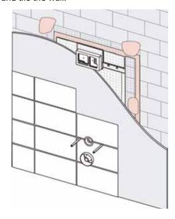
The wall construction must be at least 18 mm if the actuation is located on the wall (A). A minimum of 30 mm is required to install the TECEsquare II (B) and when using the flush-mounted installation frame (C).
