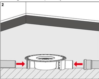
Position drain and connect to the wastewater pipe. In the case of drains with a vertical socket, a core hole with a diameter of 130 mm is required.
