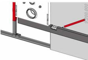
Transfer the top and bottom markings to the panel plates.
