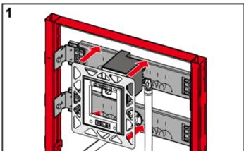
To do this, place the installation frame over the urinal barewall protection.
