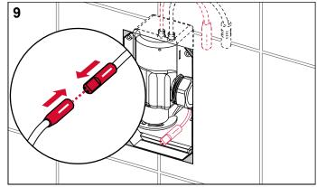
Connect the transformer's plug-in connection.
