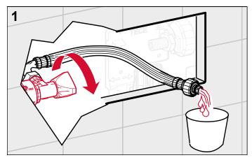
Open the corner valve and sufficiently flush out the pipe.
