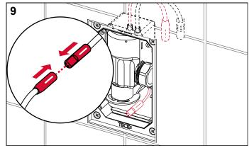
Connect the transformer's plug-in connection.
