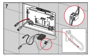
Then, insert the splash guard with the actuation motor. The activation hooks must fit correctly in the drain valve's drawbar eyelets. Tighten the splash guard clamping screws. Connect the cable from the switch on the safety support arm to the electronics (terminal strip). Ensure correct polarity.
