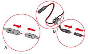
Connect the electronics to the actuation motor and the 12 V mains via the plug or terminal strip. If installed correctly, directly after connecting all plugs and the power supply, the electronics will automatically activate the motor once.
