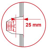
Screw in both attachment rods – distance of attachment rods to wall surface = 25 mm.
