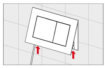
The installed cover can be detached from the flush plate using a screwdriver. To do this, insert the tool into the recesses on the underside of the flush plate and carefully remove the cover.
