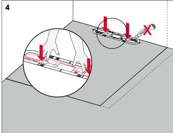
After cleaning the screed (vacuuming, brushing), push down with your fingers on the areas marked with "push" on the inner part of the protective cap. This will separate the inner area from the external area of the protective cap.
