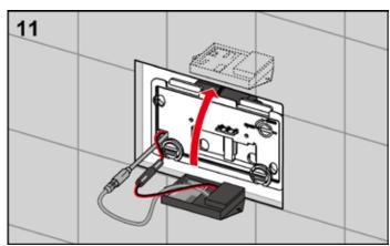
Install the electronics on the cistern or in another suitable location in the wall. Finally, install the flush plate.
