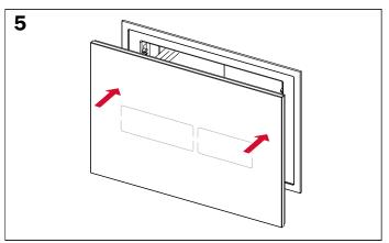
Mount the glass cover of the TECElux Mini electronics.
