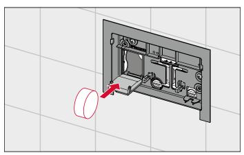
The tablet can now be placed in the insert chute through the red flap. The tablet falls into the collector basket from where it releases its active ingredients into the water.
