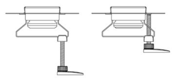
Height-adjustment facility of the assembly feet
