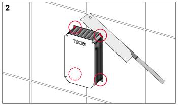
Use a saw to cut the corner areas, where the wall is thicker, flush to the wall.
