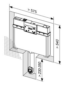
If the flush pipe (made of PE) is too long for the arrangement, it must be removed from the cistern and cut to length (maximum 120 mm).
