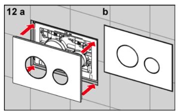
Allow the TECEloop flush plate cover to click into place in the support frame.
