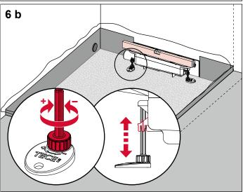
Adjust the height of the assembly feet, align horizontally and place in the indentations in the sound insulation strip. The height of the top edge of the drain must correspond with the later top edge of the screen.
