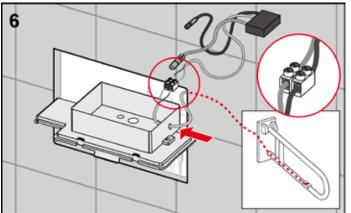
Open the cistern cover and remove it with the installation box. Guide the cable from the switch on the safety support arm from the side into the box and connect it to the electronics (terminal strip – ensure correct polarity).
