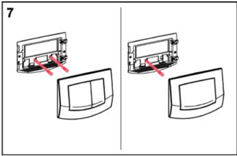
For dual-flush technology, two actuating rods (red and grey) are installed, whereas just one (grey) is required for single-flush technology.
