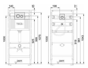
Toilet flush plate (left) and urinal flush plate (right) with 1120 mm module
