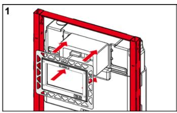
To do this, place the installation frame over the polystyrene bare-wall protection.
