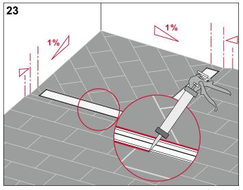
Seal the joint between the stainless steel channel and the tiles or natural stone with permanently flexible material.
