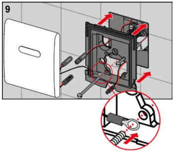
Earth the electronics via the fastening screw on the flush valve housing (see details) and screw the support frame onto the urinal flush valve housing.
