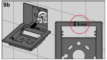
Screw in the actuating rods as described above (for the wall-mounted TECEloop, distance to wall surface = 9 mm) and screw on the counter nut to prevent them from turning. The setting length for the actuating rods is indicated on the top of the support frame. This enables you to set the rods quickly and easily.
