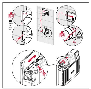
The reinforced hose and the electrical cable which are located in the lower part of the module, can be used at any time to connect the shower toilet. In the assembled state, the ceramic covers the water and power connections.
