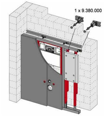
Installing the module for the safety support arms and support systems with a flushmounted profile in front of a solid wall
