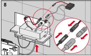
Then connect the electronics first to the motor (grey plug) and then also to the batteries (black plug). If the installation is correct, the motor will be activated once for checking purposes.
