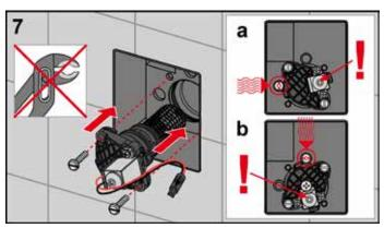
Install the electric cartridge (do not insert with tool !) and tighten the screws by hand.
