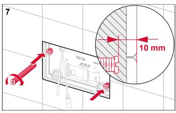
Screw in both attachment rods – distance of attachment rods to wall surface = 10 mm.
