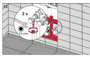
Screw in both corner valves and screw the enclosed reinforced hoses onto the corner valves.
