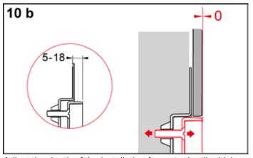
Adjust the depth of the installation frame to the tile thickness (5–18 mm). If the wall structure is thicker (up to 33 mm), as is the case for example with natural stone, you can use a suitable upgrade kit (order no. 9820181).
