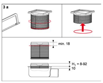
The drain top must be cut to length, the O-ring seal should sit in the lowest groove.
