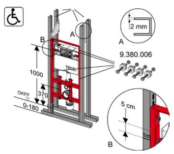
Module attachment with installation in a floor-to-ceiling UA-profile metal stud wall
