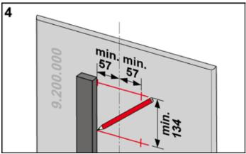
Mark the dimensions of the inside of the installation frame - width 114 mm, height 134 mm - in the centre of the plasterboard.
