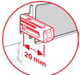
Screw in both actuating rods – distance to front edge of support frame = 20 mm.
