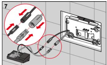
Connect the radio electronics first to the motor (grey plug) and then also to the batteries (black plug). If the installation is correct, the motor will be activated once for checking purposes.
