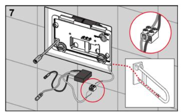
Connect the cable from the switch on the safety support arm to the electronics (terminal strip). Ensure correct polarity.
