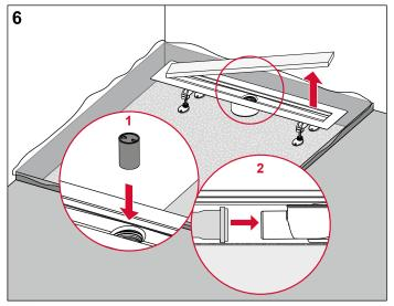
Remove the protective cover, insert the immersion pipe and attach the drainage pipe to the outflow nozzle.
