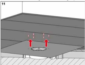
Insert pins for flange assembly (6 x).
