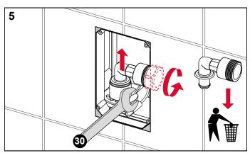
Loosen and remove the flush pipe elbow.
