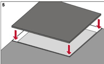
Cut the sound insulation mat to size and lay in place.
