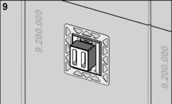
Remove the protective foils from the bonding surfaces on the installation frame, and stick them, together with those of the support frame, onto the plasterboard. Observe the correct position of the "TOP" marking, and ensure horizontal alignment.
