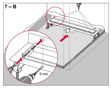
... Attach the channel to the wall. Remove the wall attachment screws again after the screed has hardened.
