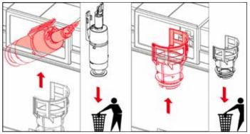
The old A1 drain valve should be disposed of, together with the associated valve seat and seal.
