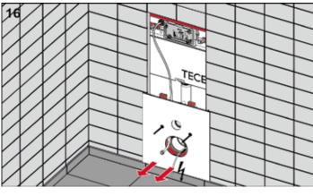
Guide the reinforced hose and power cable through the sewage water connection opening in the glass attachment facing.
