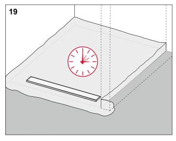
Allow the composite seal to harden, observe the specified drying time.
