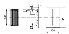
Dimensions of plastic urinal electronics and bare-wall protection for vertical slot alignment
