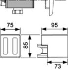
The flush valve housing is inserted into a slot in the wall and attached using a holding plate. The water connection and the intake for the urinal ceramics can be installed using any approved piping system.
