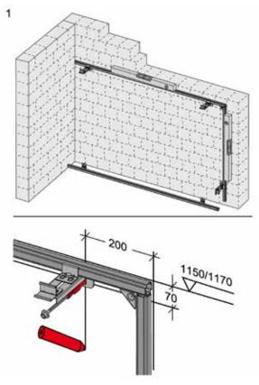
Secure the section tube to the wall with double joints, and to the floor with angle brackets
