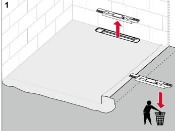
After the wall covering has been applied, the shower profile can be installed. To do so, remove the protective cap from the drain.
