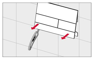
The installed cover can be detached from the flush plate using the disassembly tool. To do this, insert the tool into the recesses on the underside of the flush plate and carefully remove the cover.
