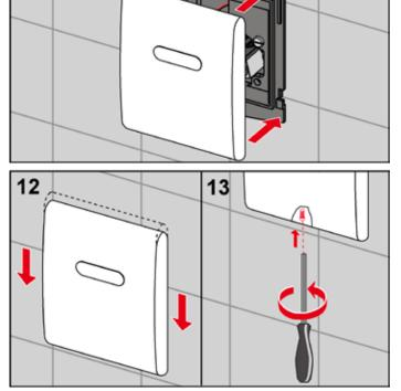
Finally, install the flush plate cover and mount the vandal-resistant screw supplied.
