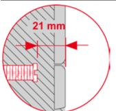
Screw in both attachment rods – distance of attachment rods to wall surface = 21 mm.
