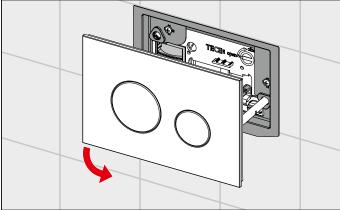
To remove the flush plate, simply take hold of the back of the plate and swivel it downwards.
