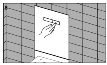
Lift up the glass facing and carry out a function test on the flushing system.
