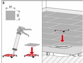
Cut the floor covering (approx.  $83 \times 83$  mm) and bond to the support with flexible adhesive (e.g. silicone or epoxy resin adhesive). After drying, insert the tile base into the grate frame.
