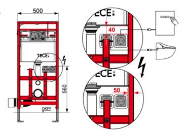
Positioning the socket(s) on the TECElux module
