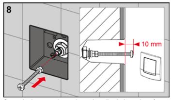
Screw in the actuating rods as described above (e.g. for the TECEambia, distance to wall surface = 10 mm), and screw on the counter nut to prevent them from turning.
