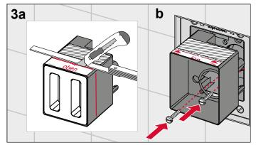
Replace the polystyrene support to provide stability, and cut the bare-wall protection along the marking. Replace the bare-wall protection and screw it onto the flush valve housing.
