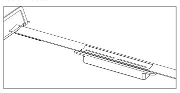
A simple height setting allows you to adjust the profile to various thicknesses of wall and floor tiles.
