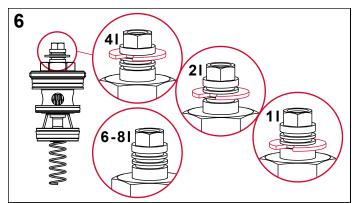
If applicable, set the flush volume before mounting the cartridge (factory setting = 2 litres). To do this, remove the retaining ring and insert it back into the corresponding slot: the first slot corresponds to a flush volume of 1 litre, the second to 2 litres, and the third slot to a flush volume of 4 litres. Without a retaining ring, the flush valve will flush a volume of 6-8 litres.
