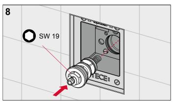
Screw in the mechanical cartridge.
