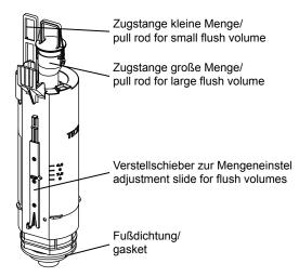
A2 drain valve, important components
