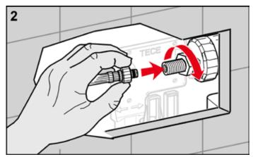
Turn the corner valve to close it again and connect the reinforced hose to the filling valve. If necessary, you can open the corner valve again.
