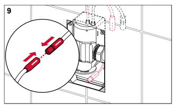
Connect the transformer's plug-in connection.
