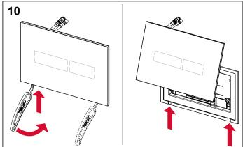
The cover can be detached from the flush plate using the disassembly tool. To do this, insert the tool into the recesses on the underside of the flush plate and carefully remove the cover.
