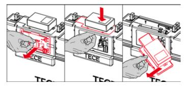
Electric socket for wiring up on the tank top, can be taken out from inside
