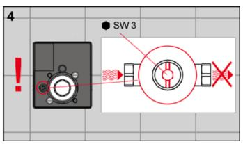
Before mounting the cartridge, ensure that the inlet flow control is closed so that no water can leak out during assembly. Close the shut-off using an Allen key. In the free-flow setting (fig. 3), the shut-off slot is parallel with the housing, and in the closed setting (fig. 4), it is at right angles to the housing.
