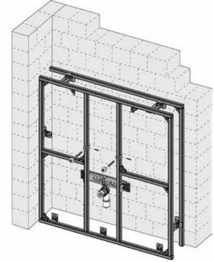
Individual construction with connection unit for washstand
