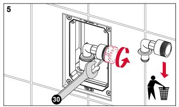
Loosen and remove the flush pipe elbow.
