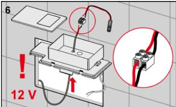
Open the cistern cover and remove it with the installation box. Guide the cable from the transformer through the bottom opening and connect it to the mains connection adapter (ensure correct polarity – see details in fig. 6).
