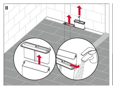
The odour traps can be pulled out using the stainless steel brackets. To clean them as quickly as possible, the traps can simply be pulled apart and cleaned with water and a cloth.
