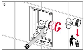
Loosen and remove the flush pipe elbow.
