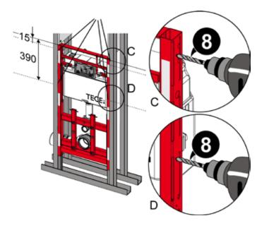
Mounting holes must be drilled to attach the module
