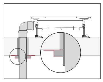
In the event of fire, the foaming material inside the fire protection sleeve expands with strong foaming pressure, permanently closing the opening in the component and preventing the spread of fire and smoke.
