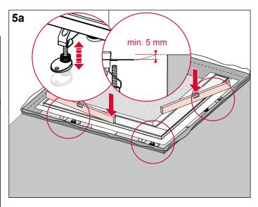
Use the adjustable assembly feet to raise the shower channel to the required position and align horizontally.
