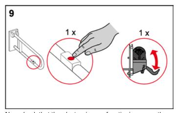
Now check that the electronics are functioning correctly: To do this, press the button again to activate the motor (once).
