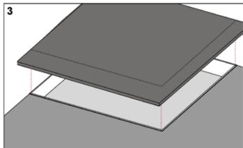
Transfer the required dimensions to the "Drainbase" sound insulation mat.
