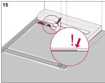
Apply the first coat of composite seal. In doing so, completely work in the Seal System sealing tape and corners.
