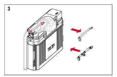
Remove the reinforced hose and mount the replacement reinforced hose in reverse order.
