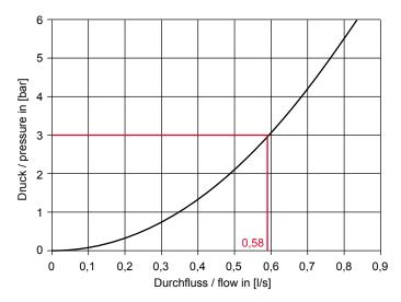
Flow diagram of urinal electronics
