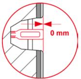
Turn both actuating rods until they are in contact with the surface of the wall.
