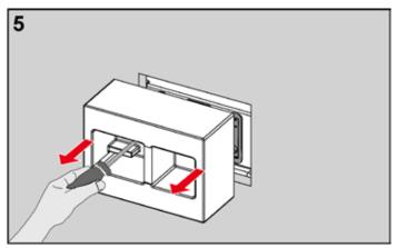
Remove the protective foils from the bonding surfaces on the installation frame, and stick them, together with those of the support frame onto the plastered surface. Observe the correct position of the "TOP" marking, and ensure horizontal alignment.
