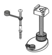
Sound-absorbing element on assembly foot
