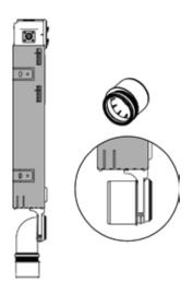
Two-part drain bend – also for horizontal connection
