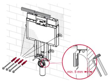
Attach the water connection (connection R 1/2" on cistern). Brick the module in completely and follow the outline. Install the polystyrene bare-wall protection, the threaded rods and the odour traps.
