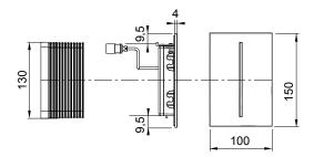
Dimensions of metal urinal electronics and bare-wall protection for vertical slot alignment
