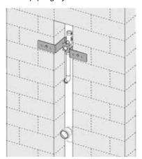
The urinal flush valve is locked in its as-delivered state so the required pressure test can be performed.
