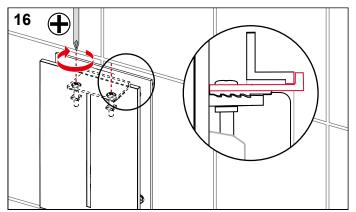
Mount the anti-theft device from the top of the cover using a Philips screwdriver.
