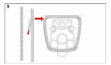
Mount the sound insulation strips on the ceramic.
