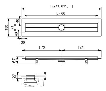
Straight channel body for installation in screed, with flange and Seal System\* sealing tape, for creating a tested and certified connection of the TECEdrainline channel to the composite seal.
