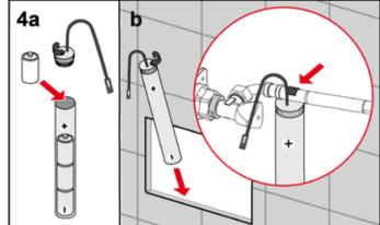
Place the four batteries in the housing and hang the waterproof battery compartment on the reinforced hose in the cistern.
