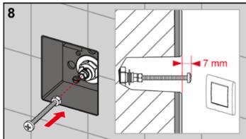
Screw in the actuating rods as described above (for the wall-mounted TECEplanus, distance to wall surface = 7 mm) and screw on the counter nut to prevent them from turning.
