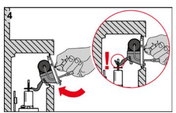
Insert the (new) splash guard for the electronics with the actuation motor. The activation hooks must fit correctly in the drain valve's drawbar eyelets. Tighten the splash guard clamping screws.
