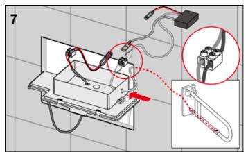
Guide the cable from the switch on the safety support arm from the side into the box and connect it to the electronics (terminal strip). Ensure correct polarity.
