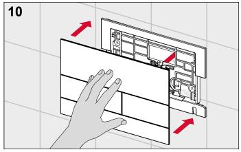
Allow the TECEsquare II flush plate cover to click into place in the support frame.
