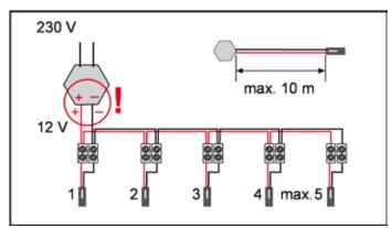
Connect the transformer cable to the mains connection adapter. Ensure correct polarity when making the connections
