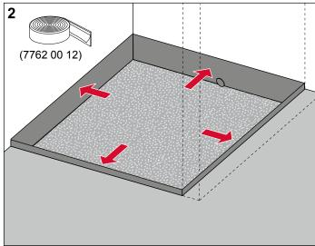
Apply the edge insulation strips.
