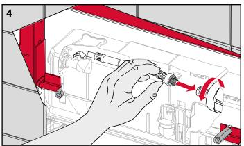
Remove the splash guard, sufficiently flush out the connecting pipe and screw onto the filler valve.
