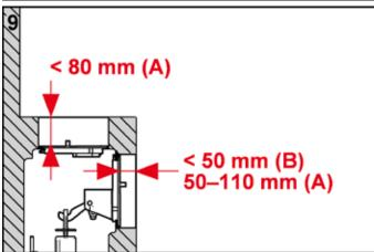
Break off the actuating rods according to the wall structure.
