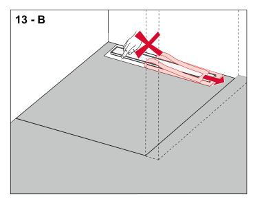
Completely remove the protective sheet from the channel flange. Do not touch the flange any more or let it get dirty.
