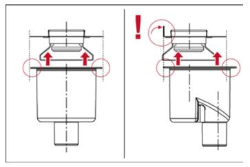
When installing the channel against the wall, the flange must be flush with the edge of the drain.
