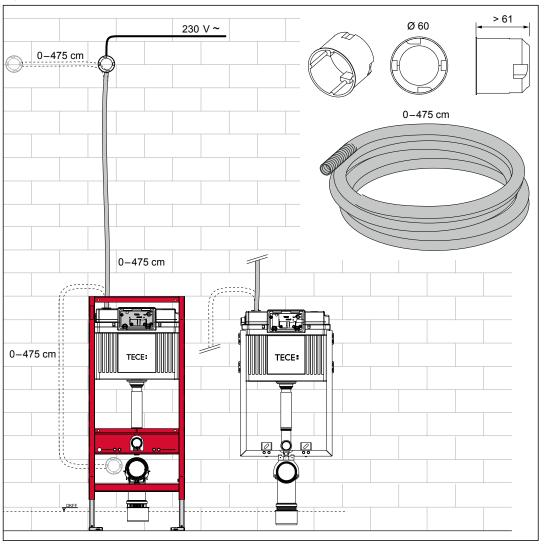
Positioning the transformer: In the 0-475 cm range around the cistern (entire cable length: 5 m).
