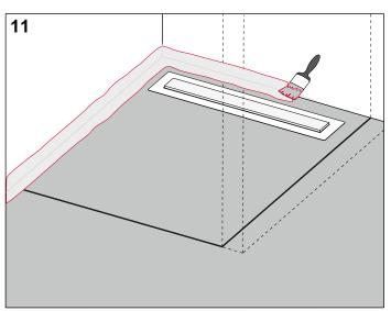
Apply a coat of composite seal to the transitions between the wall and the screed. Observe the manufacturer's instructions when creating the composite seal (figs. 11 to 19).
