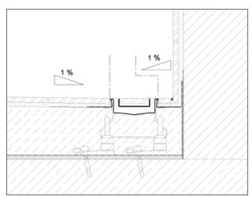
Installation "close to the wall", incline
