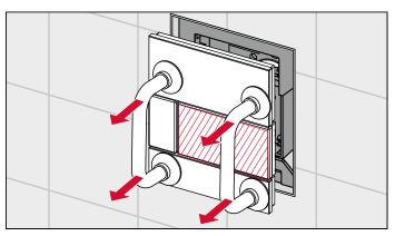
When mounting or dismounting the cover, do not press the button. The installed cover can be removed from the flush plate using the bow-type handles included in the installation frame's scope of supply. Only position the suction cups on the cover to be removed.
