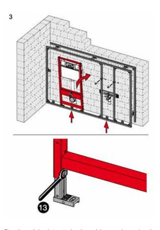
Place the angle bracket centred on the module or crossbeam, place the module feet onto the section tube, and release the foot brake
