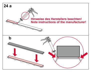
Stick the adapted covering with suitable adhesive onto the support sheet (following the manufacturer's instructions). Seal the space between the bonded covering and the support with permanently flexible material.
