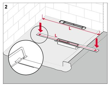
If the existing width of the shower zone does not correspond exactly with the as-delivered lengths of the Drain-profile shower profile, the profiles can be shortened with a saw. This should only be done with a stainless steel saw blade. The saw blade should be unused or it should at least be ensured that it has never been used to cut ferrous productions (steel, etc.). Otherwise, ferrous ions could be introduced causing external rust on the stainless steel profile.
