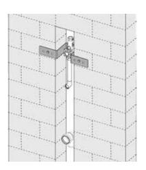
In the as-delivered state, the urinal flush valve is locked, so that the required pressure test can be carried out. The inlet flow control is located above the plug. It must not be removed until the fine installation phase.
