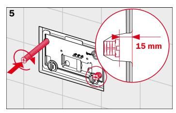
Screw in both attachment rods – distance of attachment rods to wall surface = 25 mm.
