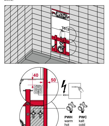
Position of socket and corner valve with TECEone
