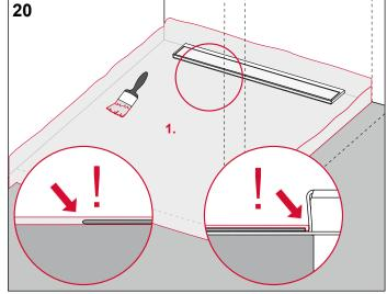
Apply the first coat of composite seal spotlessly over the entire area. In doing so, fully integrate the Seal System sealing tape.
