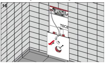
Guide the reinforced hose through the top cut-out in the glass facing.
