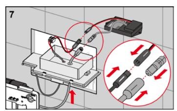
Connect the radio electronics first to the motor (grey plug) and then also to the batteries (black plug). If the installation is correct, the motor will be activated once for checking purposes.
