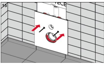
Mount the lower glass attachment facing and — if not already carried out at the factory — insert both glass protection caps.
