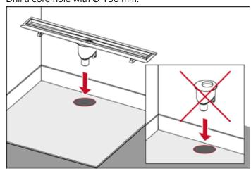
Insert the drain body including the drain channel into the core hole. Check for leaks. The edge of the drain must be packed with screed – make sure that there are no cavities.
