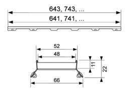
Dimensions of "plate II" tileable channel
