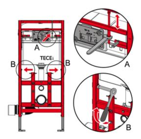
If a toilet ceramic is already mounted, slightly loosen the nuts attaching the ceramic.
