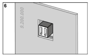
Screw the plasterboard centrally over the module.
