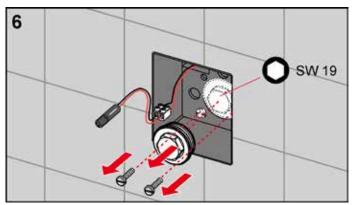
Remove the bare-wall plug and unscrew the fastening screws on the bare-wall protection.
