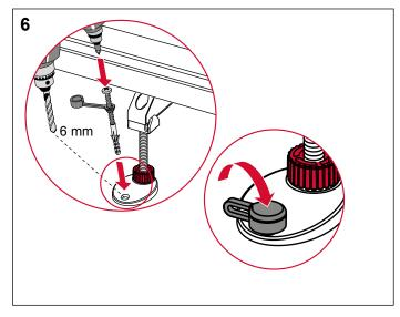
Fasten the assembly feet and press sound insulation caps onto the bolt heads.
