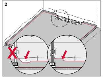
Make sure that the drain fits flush with the screed without any cavities.
