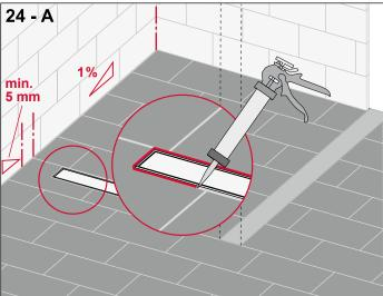
If necessary, also seal the wall areas with composite seal, following the manufacturer's instructions, and apply the tiles or natural stone covering.
