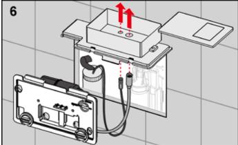
Open the cistern cover and remove it with the installation box. Guide the battery connections and actuation motor from beneath through the openings in the bottom of the box.
