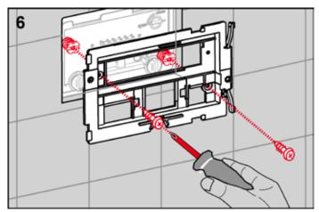
Mount the support frame to the attachment rods.
