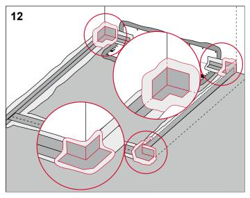
Finally, work the sealing tape and corner seals completely into the sealing material. The sealing tape should overlap the Drainprofile sealing sleeve by at least 50 mm.
