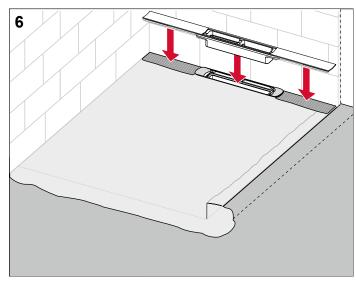
Then insert the shower profile with the supports into the drain. Also make sure, when doing so, that no tile adhesive gets into the drain (if necessary, remove any tile adhesive afterwards).
