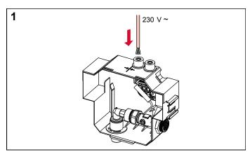
The U 2 flush valve housing can be installed in dry-walls and brick-walls. The transformer is already integrated into the flush valve housing to facilitate coordination of the different trades carrying out the assembly work. Therefore, the transformer can be directly connected with a 230 V cable.
