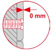
Turn both attaching rods until they are in contact with the surface of the wall.
