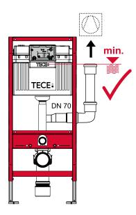
Watertight installation up to the cistern's water column
