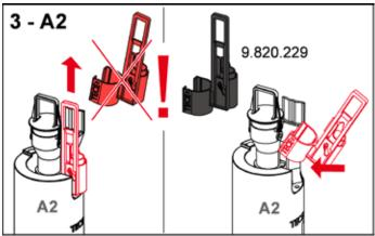
Then adjust the drain valve to the toilet electronics: on newer cisterns installed after mid/end of 2009, the red pull rod of the valve (A2) must be replaced by a black one (see figure above).
