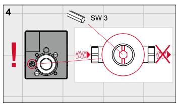
Before mounting the cartridge, ensure that the inlet flow control is closed so that no water can leak out during assembly. Close the shut-off using an Allen key. In the free-flow setting (fig. 3), the shut-off slot is parallel with the housing, and in the closed setting (fig. 4), it is at right angles to the housing.
