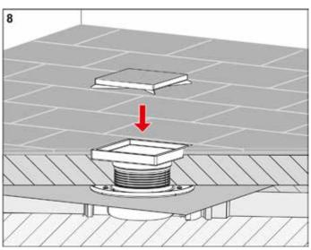
After drying, insert the tileable channel into the grate frame.
