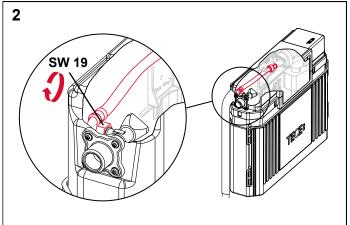
Close the corner valve in the cistern and loosen the reinforced hose including the thread connection on the filling valve.
