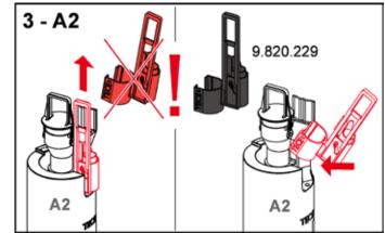
Then adjust the drain valve to the toilet electronics: on newer cisterns installed after mid/end of 2009, the red pull rod of the valve must be replaced by a black one (fig. 3 - A2).
