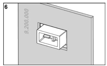
Screw the plasterboard centrally over the module.
