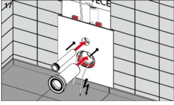
Cut the toilet connection set to a suitable length and insert.
