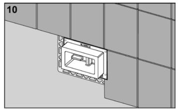
After adjusting the depth, you can tile right up to the installation frame.
