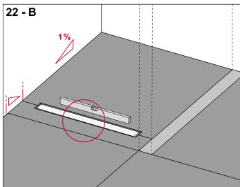
Create the cut-outs in the covering, preferably using a water jet cutter. The gap width must be between 6 and 8 mm.
