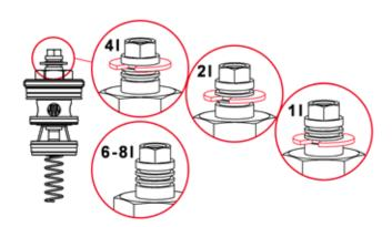
Adjusting the volume on the mechanical cartridge
