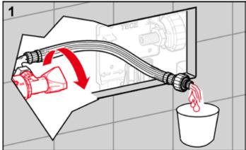
First remove the splash guard with the flush plate - this will no longer be required. Open the corner valve and sufficiently flush out the pipe.
