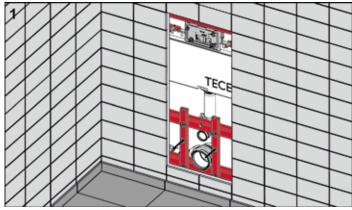
Remove the bare-wall protection.
