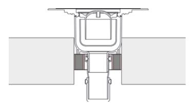
As temperatures rise during a fire, this material foams up to many times its original form. This causes the remaining annular gap towards the core hole on the outside of the fire protection sleeve to close.
