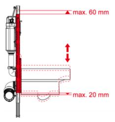
After adjusting the height, tighten the two side restraining screws back up again.
