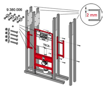
Installation in a metal stud wall
