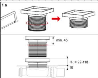
Install the drain top – it must be cut to length.
