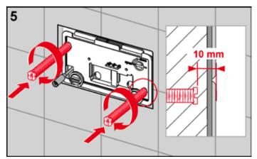
Mount the two attachment rods – distance to wall surface = 10 mm.
