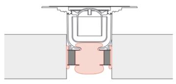
In the socket area, the outflow nozzle including the pushed-on HT pipe sleeve becomes crushed.
