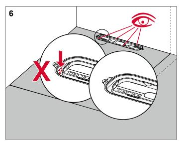
Check the groove area for dirt. Carefully remove any dirt from the groove area.
