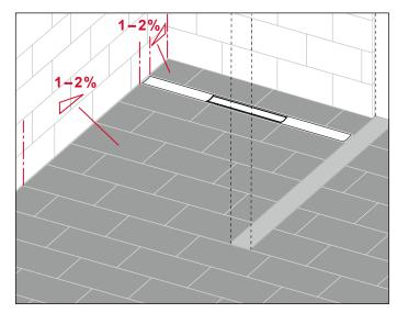
Installation "close to the wall", incline
