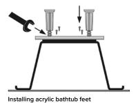
In the case of acrylic bathtubs with a thin edge, supporting the edge with additional horizontal profile braces may
