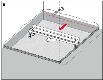
Remove the edge insulation strips above the horizontal shower flange.
