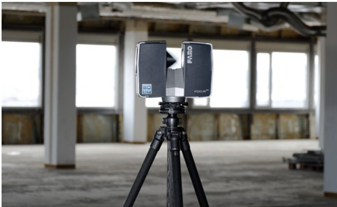
Laser scanners transform an as-built situation into a cloud of points that can be loaded into a CAD program as measurements. Measurement service providers save the bathroom builder from having to do this work. Image: www.faro.com
