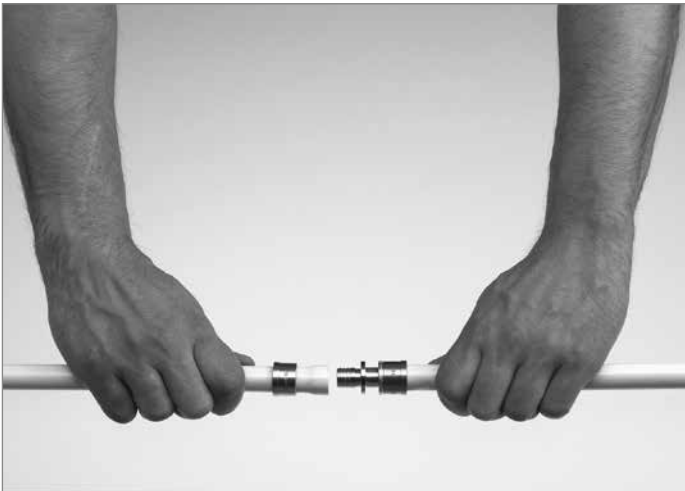
Pressing: Correct position (on left) – Incorrect position (on right)
