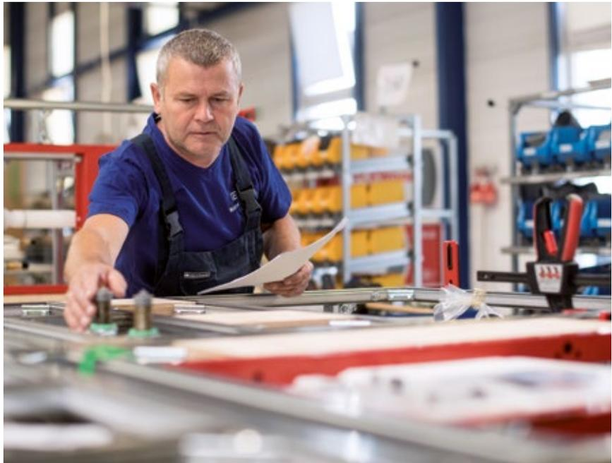
Before shipment, all assemblies are subjected to quality inspection and the multi-stage final inspection. In addition to the completeness of all fixtures, the pipe connections and insulation, we also check the respective accompanying by-pack for assembly and connection of the sanitary walls for completeness.
