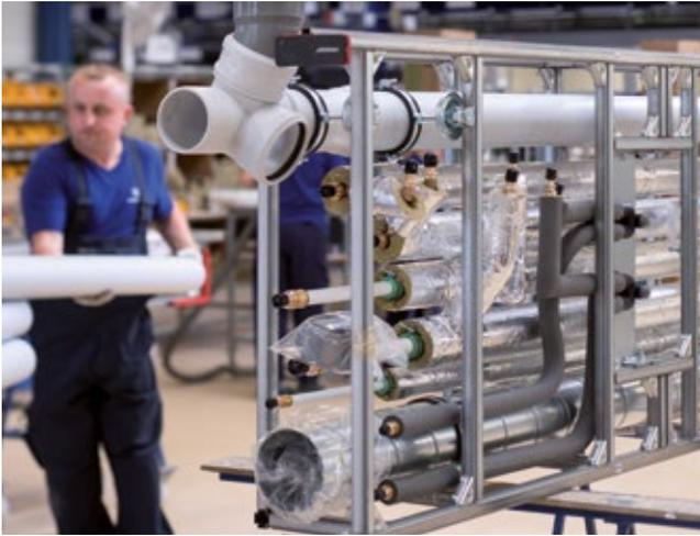
The piping for all media is then installed, sound-insulated and insulated according to requirements. The lost boarding for the ceiling filling compound is then adjusted and enclosed.
