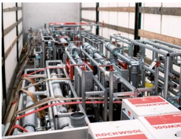
The scope of the entire cargo is then checked before the truck leaves the factory for the construction site.
