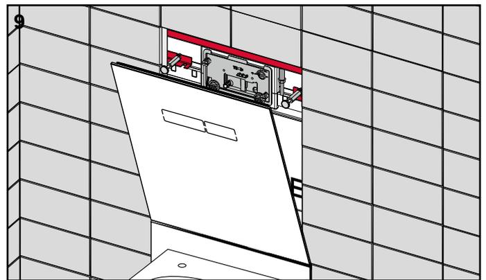
Insert the upper flush plate into the supports and lift up.
