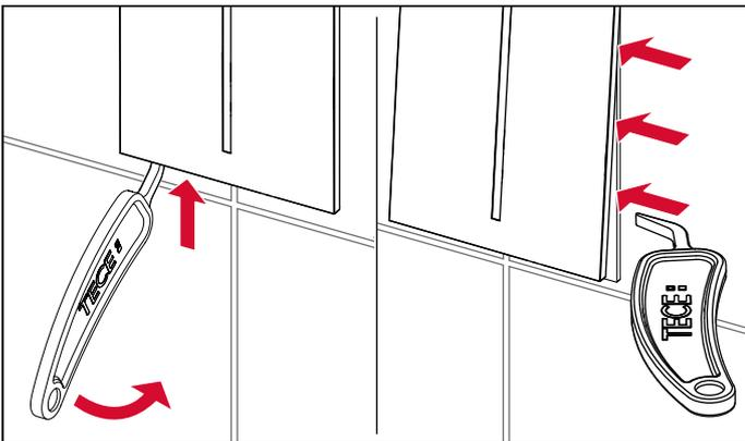
To dismantle the cover, insert the programming key into the notches on the underside of the flush plate.
