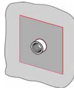
Fig. 2: Bedding the sealing collar into the still-wet sealing coating
