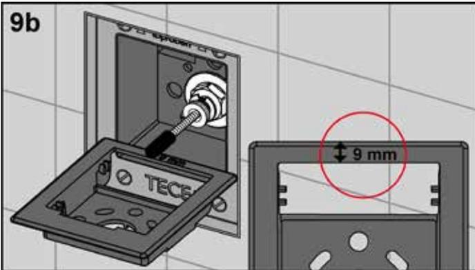
Screw in the actuating rods as described above (for flush-mounted TECEloop, distance to front edge of inside of installation frame = 9 mm), and screw on the counter nut to prevent them from turning.
