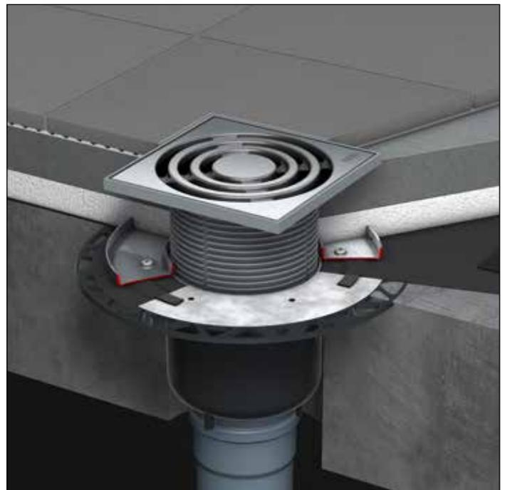
Installation in the cellar area, sealing using clamped flange sealing
