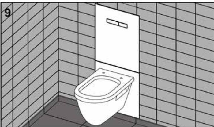
Fill the gap between the ceramic and the glass facing with permanently elastic joint sealant.
