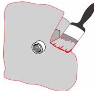
Fig. 3: Applying the upper sealing coating
