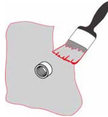
Fig. 1: Applying the lower sealing coating
