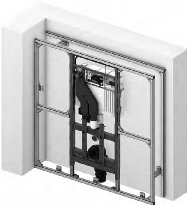
Installation in a TECEprofil pre-wall
