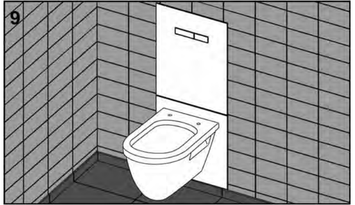
Fill the gap between the ceramics and the glass plate with permanently flexible joint sealant.
