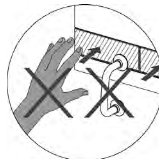
The installed cover can be removed from the actuation unit using the bow-type handles contained in the installation frame delivery.
