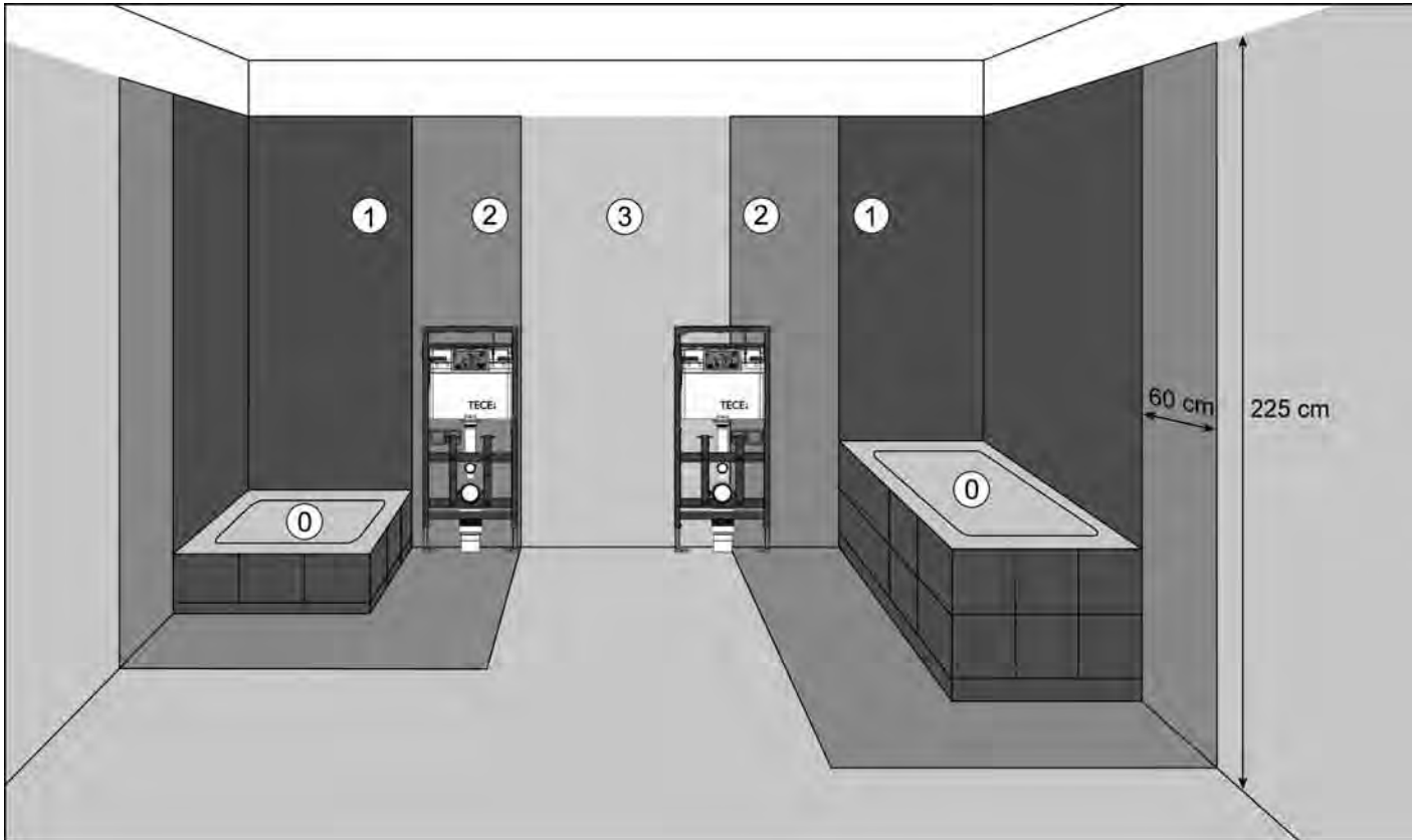
Installation of a TECElux module in protected zone 2
