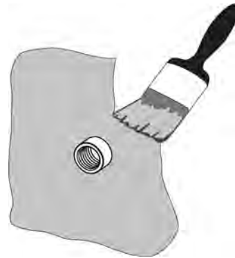
Fig. 1 Application of the lower sealing coating
