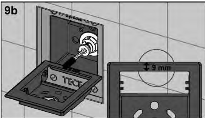
Screw the actuation rod in as far as specified (for TECEloop flush-mounted 9 mm distance to the front edge of the inner installation frame) and secure it against twisting with the lock nut.
