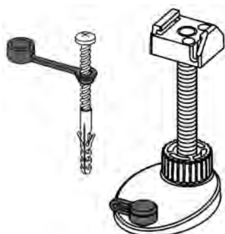
Sound-absorbing element on the mounting foot
