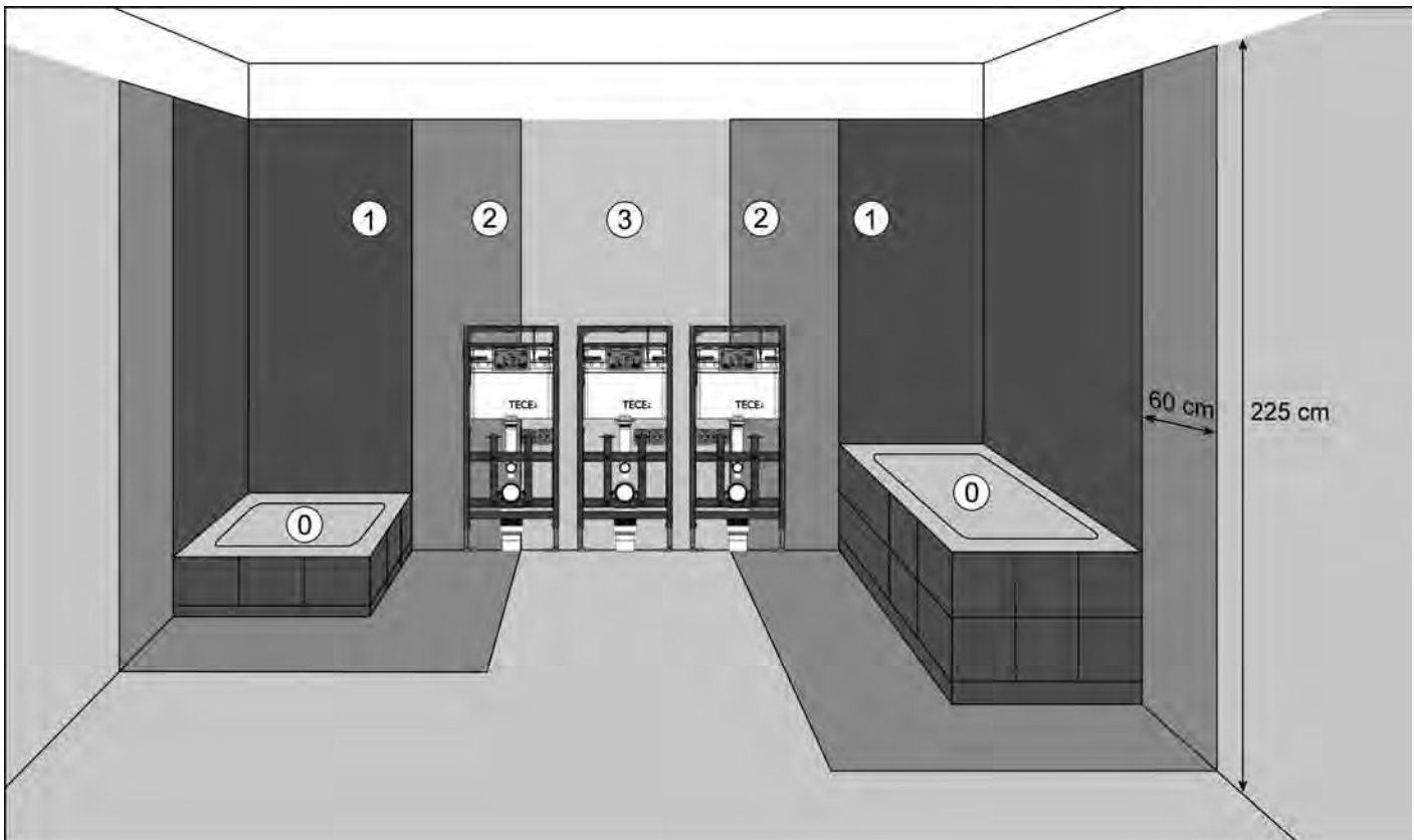
Installation of a TECElux module in protected zone 3
