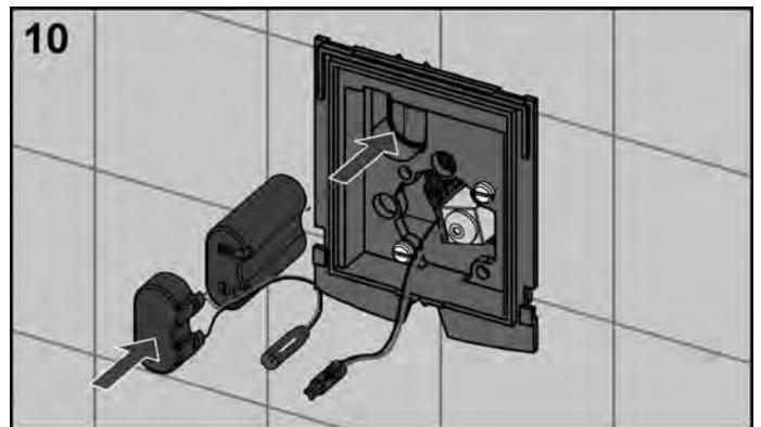
Plug the connection adapter onto the battery and position it in the opening provided.
