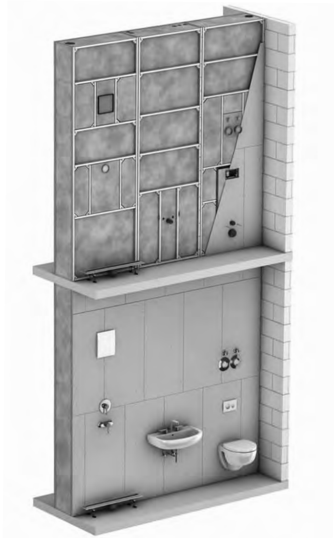
F 90 from 386 mm wall thickness
