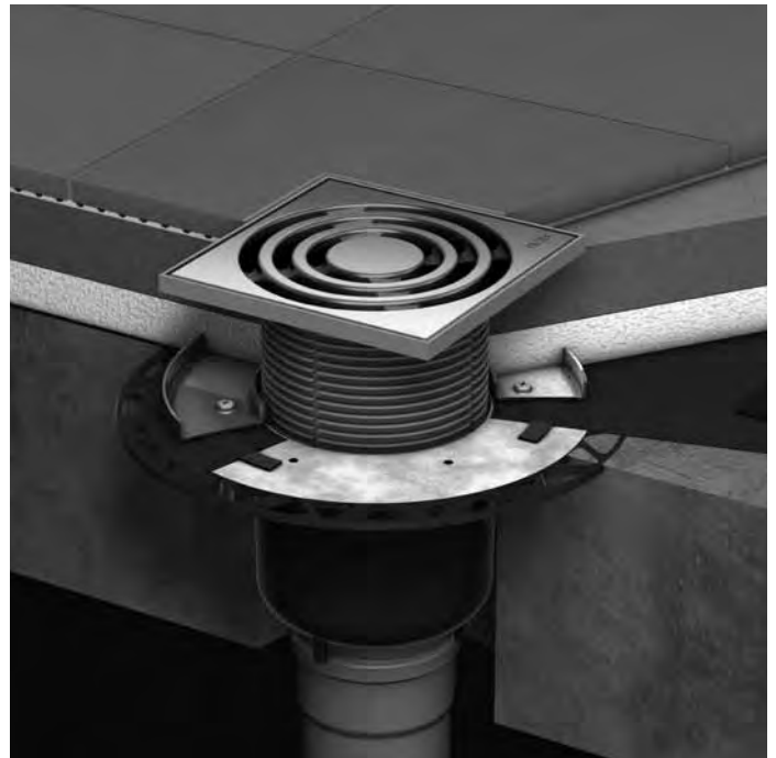
Installation in the cellar area, damp-proofing using clamped flange sealing
