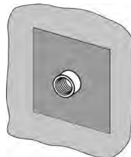
Fig. 2 Bed the sealing collar into the still-wet sealing coating
