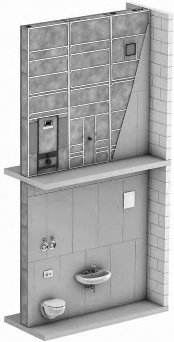
F 90 from 286 mm wall thickness
