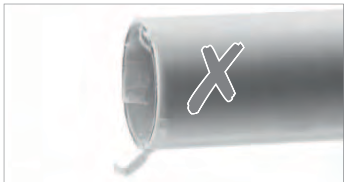
Incorrectly calibrated pipe
