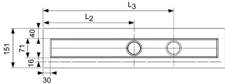
\* max. distance between outer edge of channel and drain = 750 mm
