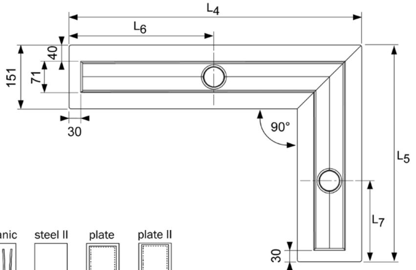
\* max. distance between outer edge of channel and drain = 750 mm
