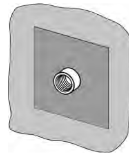
Fig. 2 Bed the sealing collar into the still-wet sealing coating
