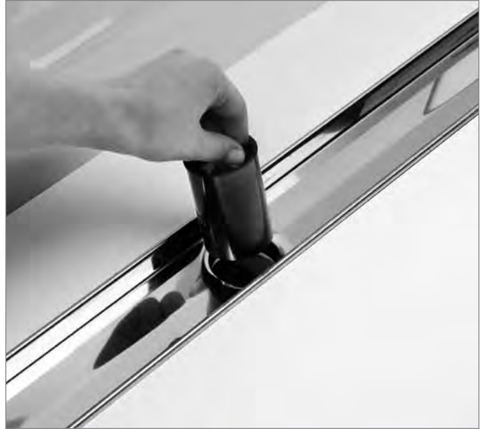
Remove the immersion pipe for cleaning purposes
