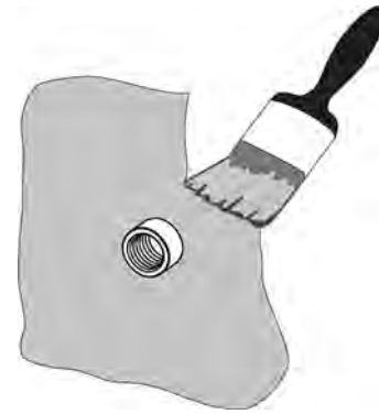
Fig. 1 Application of the lower sealing coating
