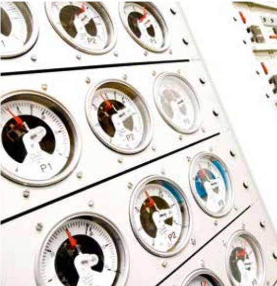
In the testing laboratory for pipe systems, points are indicated on the standard time-to-rupture curve and monitored. For instance, the service life of a pipe sample at 90°C and 10 bar is measured and recorded.
