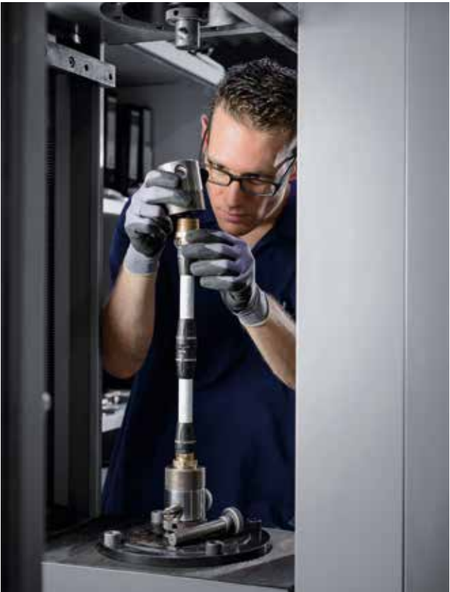
Pipes and connections undergo pull-out resistance tests to ensure maximum safety. This guarantees that the installation will remain stable in the long term.
