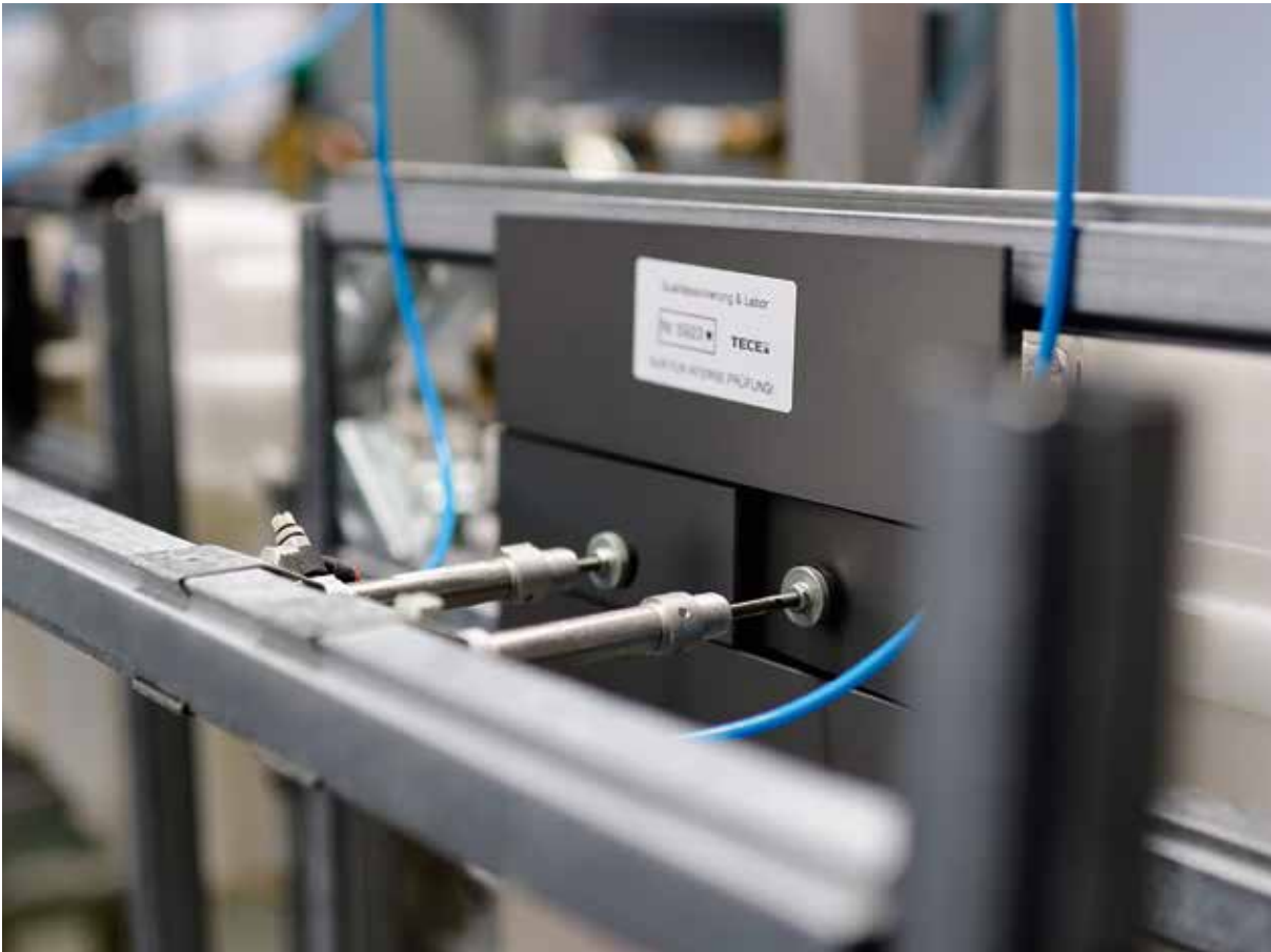
The actuation mechanism of flush plates is subjected to a 200,000-cycle fatigue test and should remain fully operational afterwards.
