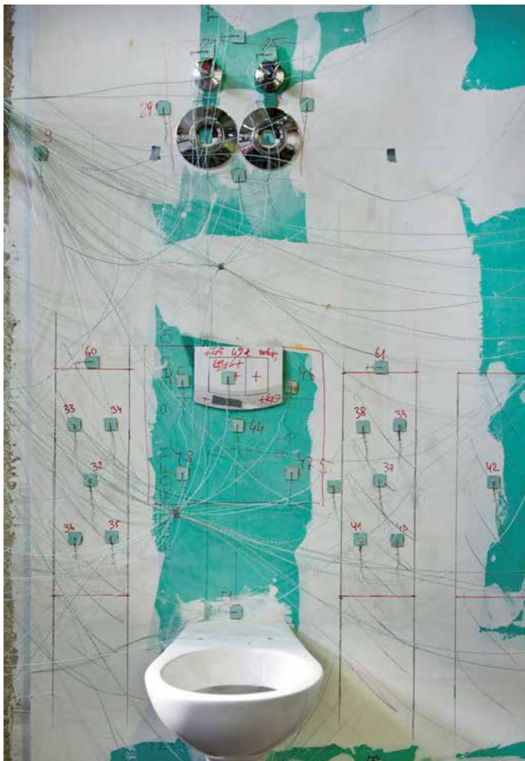
Fig. top: System for noise level measurement at the Fraunhofer Institute Stuttgart.
