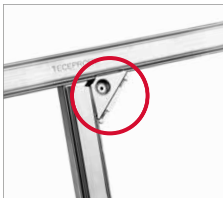
Inaccuracies (of up to 10 mm) when cutting the section tube to length can be easily rectified by the corner joint.
