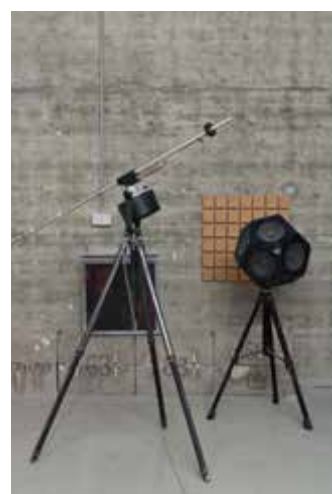
Fig. top: System for noise level measurement at the Fraunhofer Institute Stuttgart.
